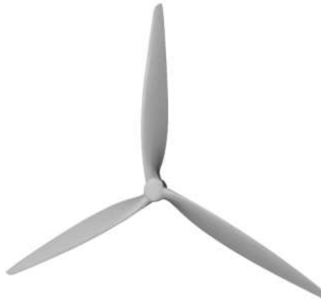
Fig. 9. Geometric model of the designed propeller for the analyzed engine-propeller propulsion system
