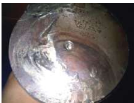
Fig. 1. Photograph of the fatigue fracture surface of the shaft (stress concentrator – thread) [1]
