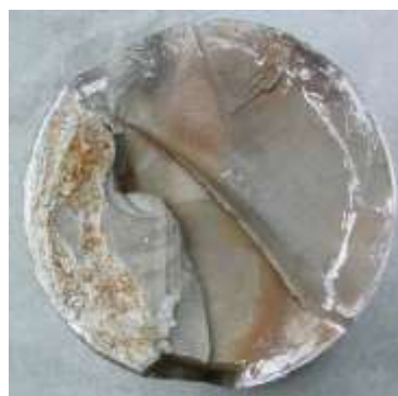
Fig. 2. Photograph of the fatigue fracture surface of the pump shaft (stress concentrator – keyway) [3]
