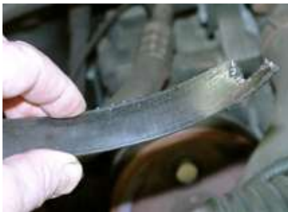
Fig. 4. Broken drive belt
