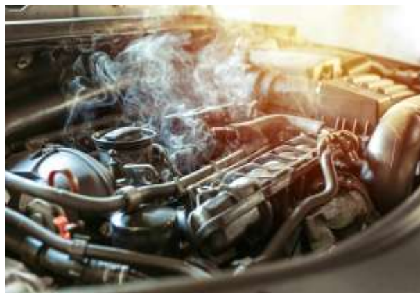
Fig. 5. Overheating of a hot engine resulting in ignition of flammable liquids
