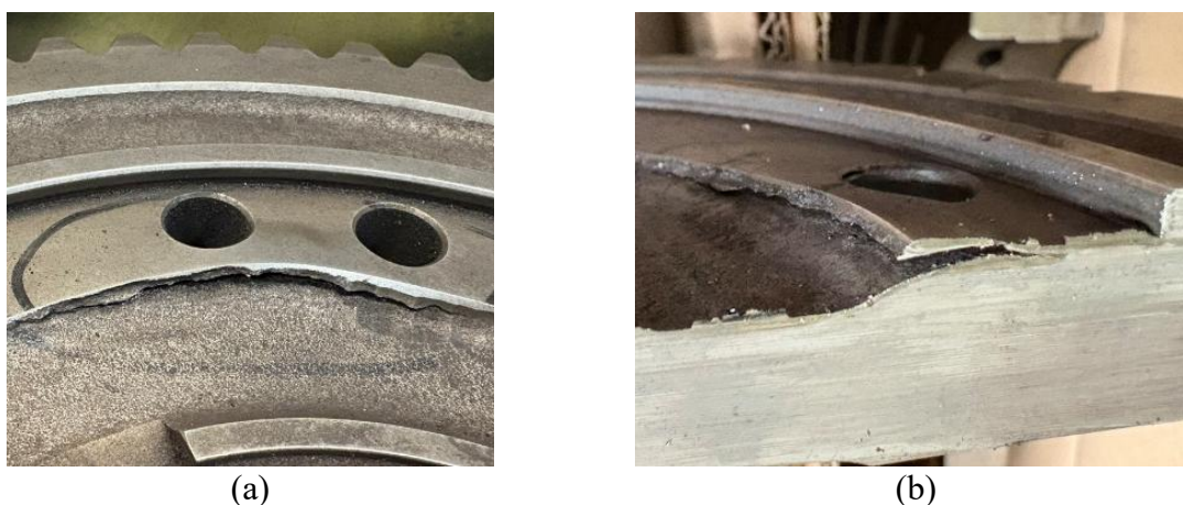
Fig. 2. Inspected forging in visual testing (VT): a) Location of cracks on forging; b) Location of cracks on forging in section
