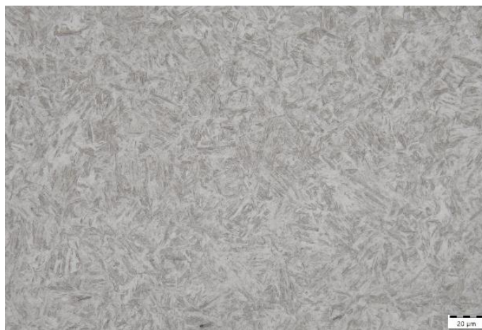
Fig. 7. Microscopic observation of the borderline structure – bainite
