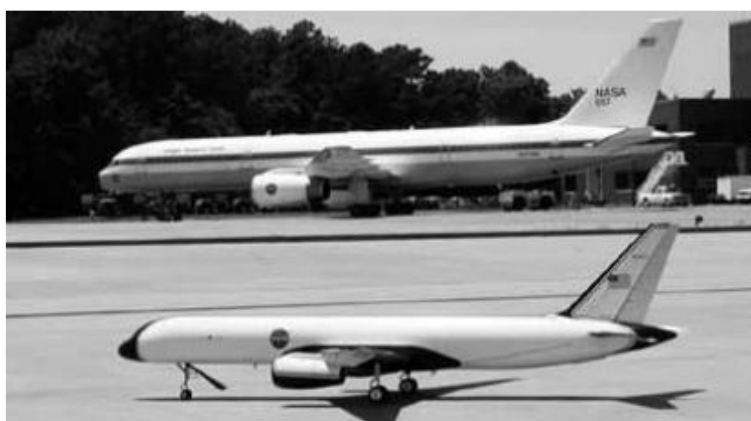
Fig. 1. Full-scale aircraft and its FDSM in AirStar NACA program
