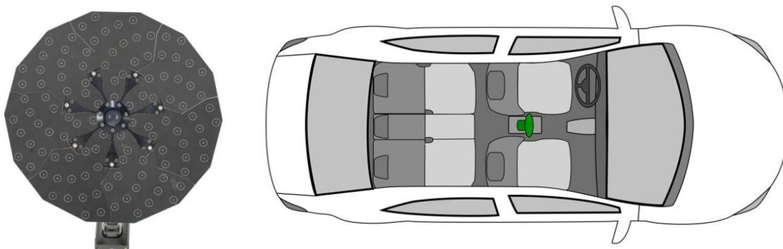
Fig. 8. View of the camera used and a diagram of the tested vehicle with the location of the acoustic camera marked in green
