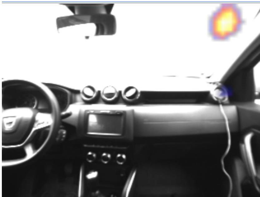
Fig. 12. Incorrect identification of the noise source
