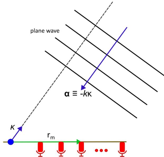
Fig. 1. A microphone array, a far-field focus direction, and a plane wave incident from the focus direction
