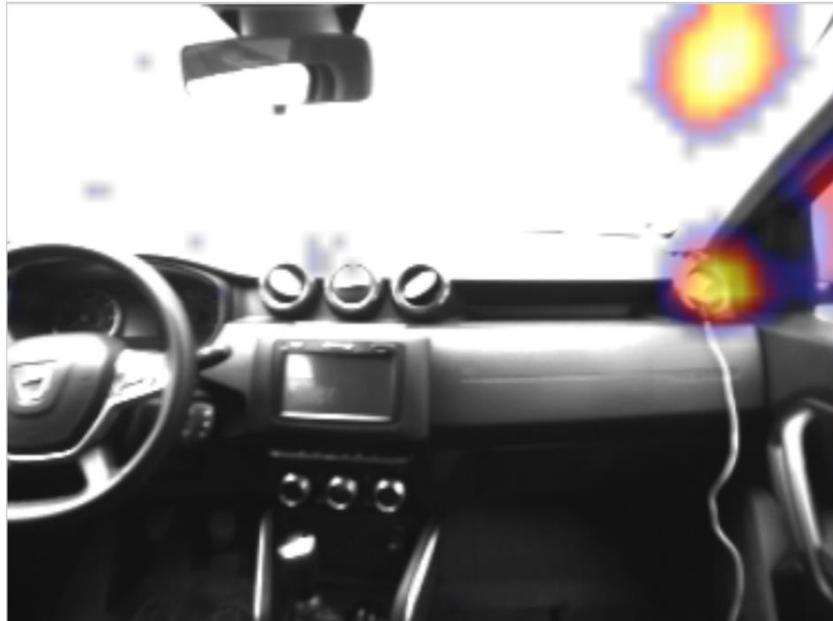
Fig. 11. Recognition of two noise sources (real and apparent)
