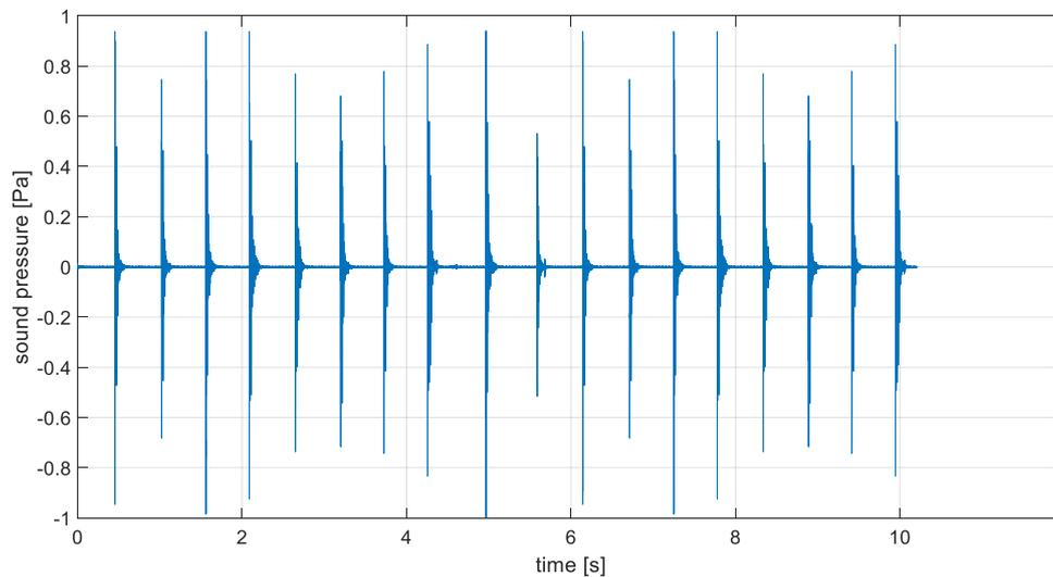
Fig. 3. Acoustic signal obtained during collisions of elements made of plastic
