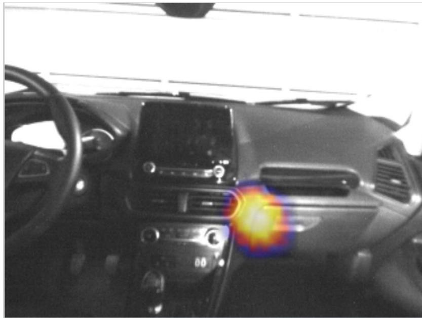
Fig. 13. Detection of the noise source during tests on the test stand
