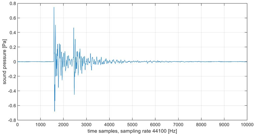
Fig. 5. An enlarged fragment of the effect of a collision between two elements of the interior of the cabin made of plastic
