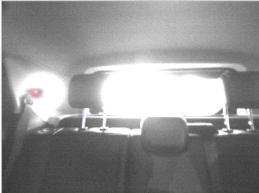
Fig. 16. Incorrect identification of the location of the noise source on the rear side window
