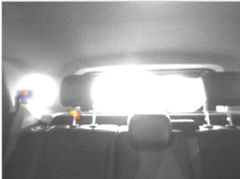
Fig. 15. The location of the noise source at the junction of the rear trunk shelf with the left rear body pillar – Result obtained during the road test
