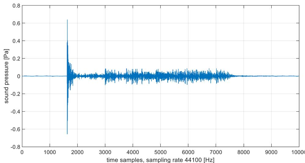
Fig. 4. An enlarged fragment of the effect of the collision of two metal elements of the interior of the cabin
