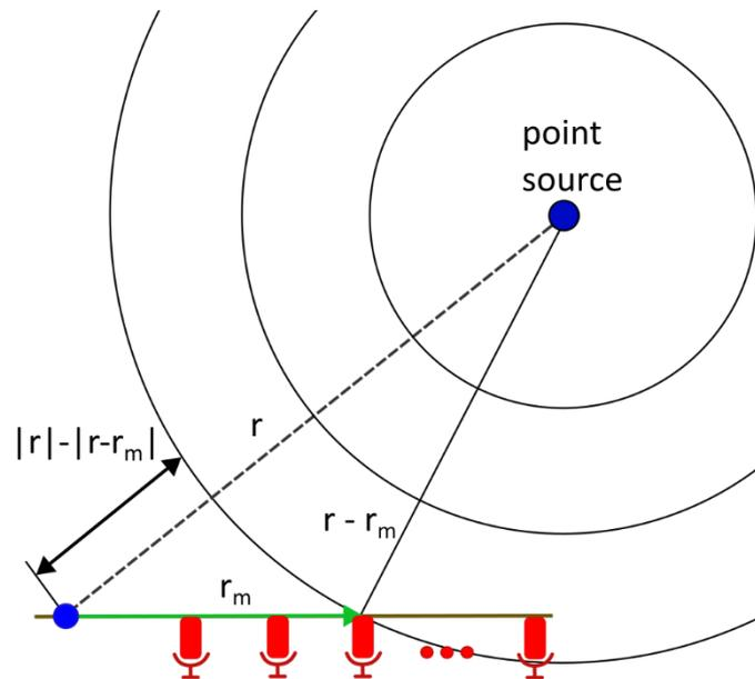
Fig. 2. In near-field focusing, spherical waves emitted by a monopole source at the focus point  $r$  are assumed
