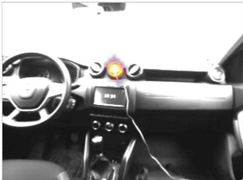
Fig. 10. Identification of the noise source located in the central air outlet
