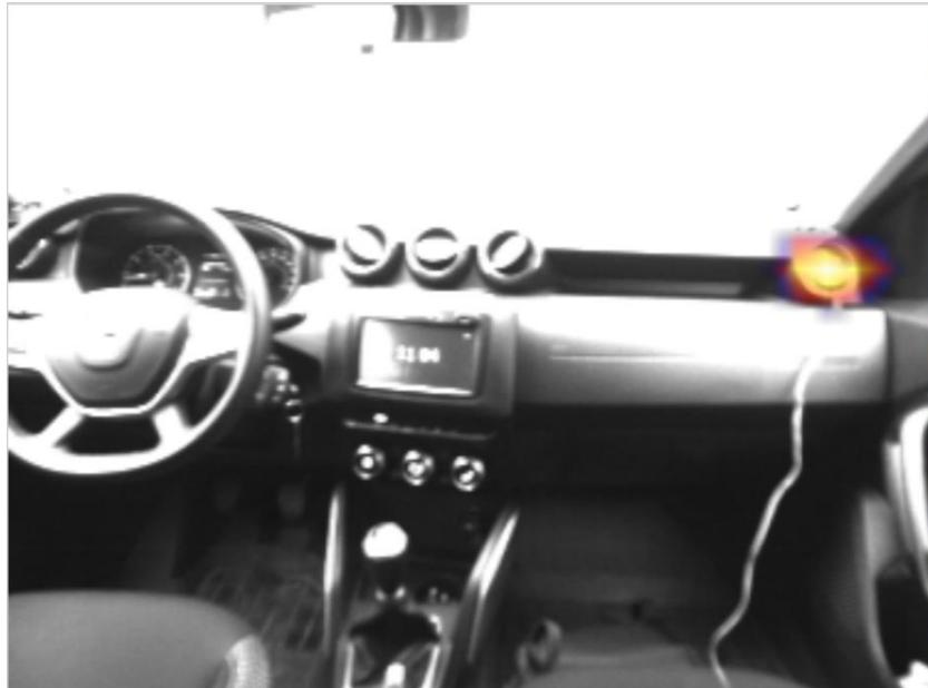
Fig. 9. Identification of the noise source located in the right air outlet
