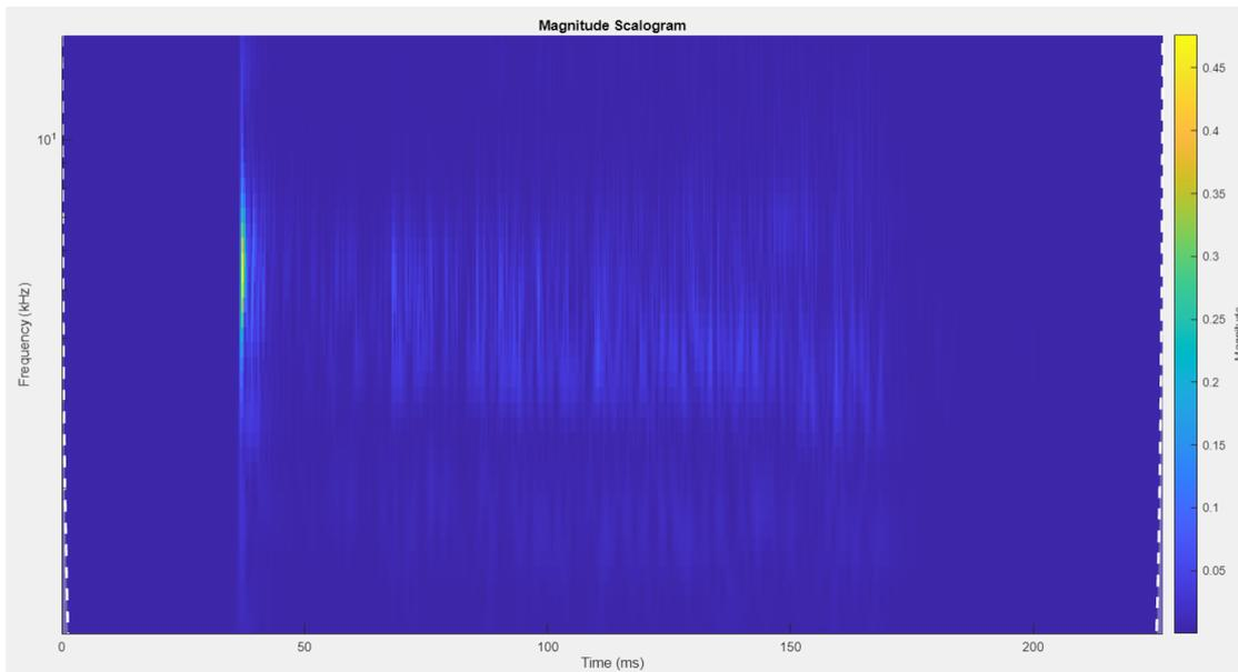
Fig. 6. Time-frequency distribution of the signal resulting from the collision of metal parts
