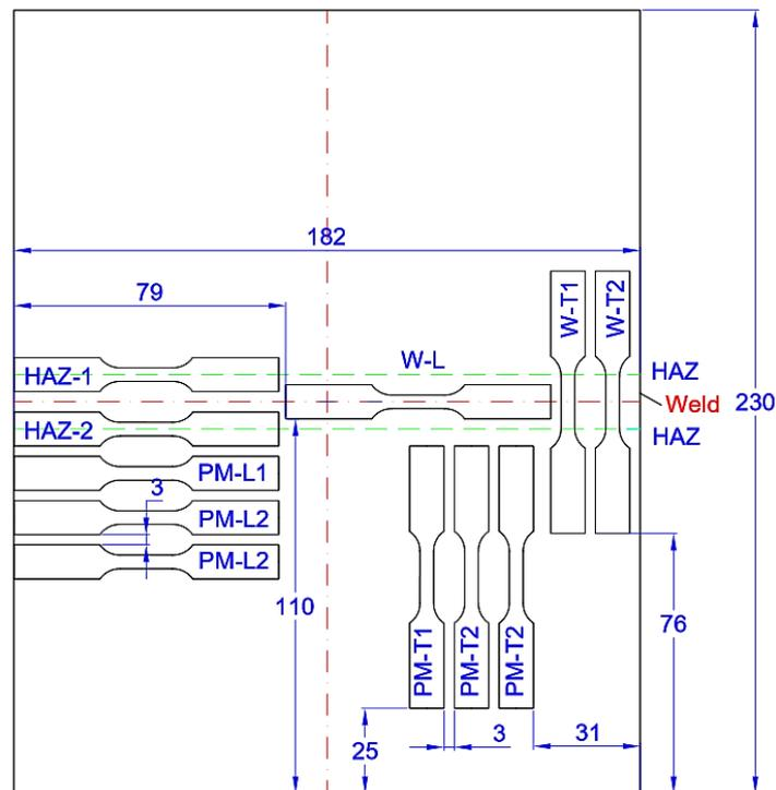
Fig. 6. The specimens' arrangements in the S700MC plate with a weld
