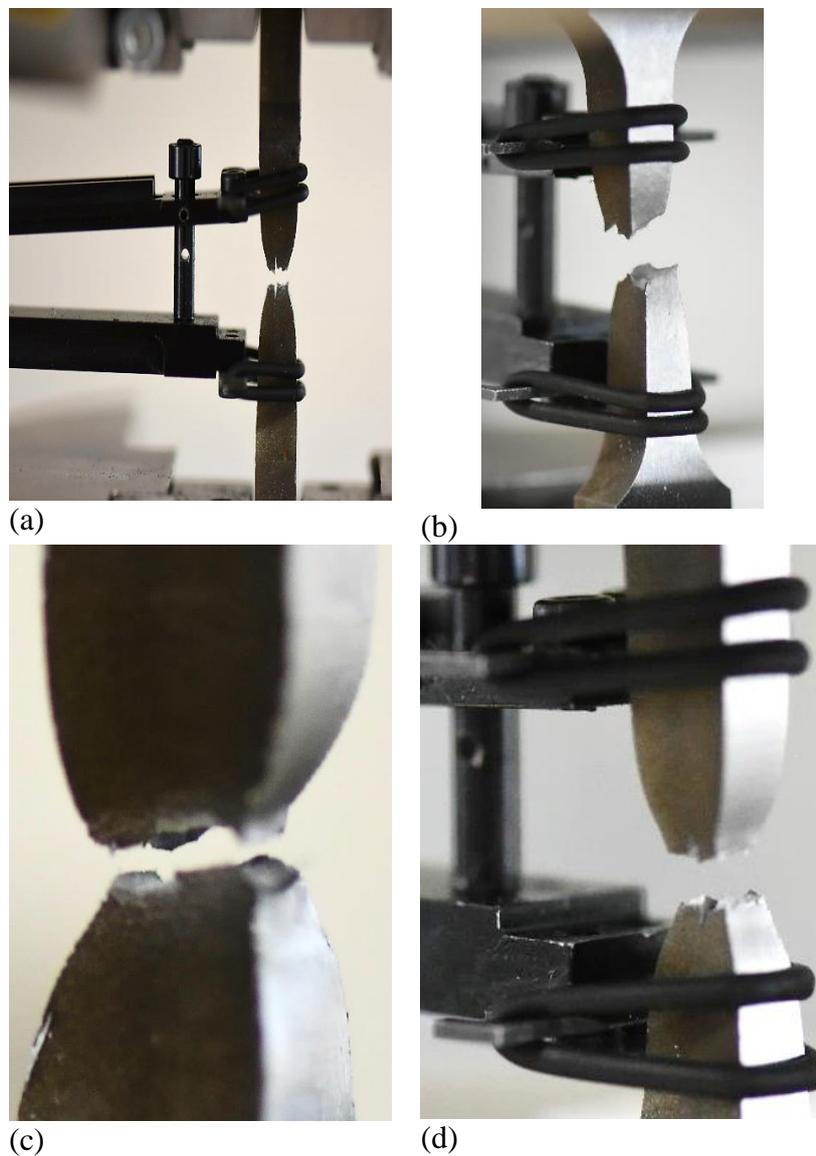
Fig. 13. Specimens after decohesion in tensile test: (a) and (b) parent material and weld in L direction - respectively, (c) weld in T direction, (d) HAZ
