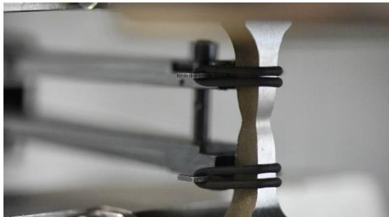
Fig. 8. Mini-specimen made of parent material (the S700MC steel) from transversal direction to the weld's major axis before the final stage of tensile test
