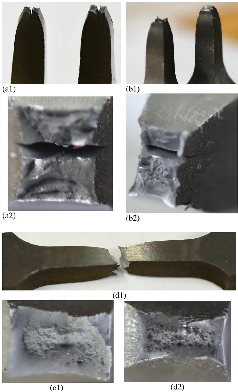
Fig. 14. Fracture zones of the parent material and weld; the parent material in (a1, a2) longitudinal and (b1, b2) transverse directions; the weld in (c1) longitudinal and (d1, 2) transverse direction
