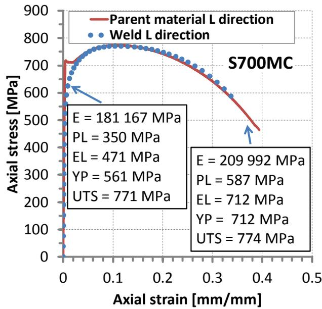
Fig. 10. Tensile characteristics of the parent material and its weld determined using specimens selected from the longitudinal direction
