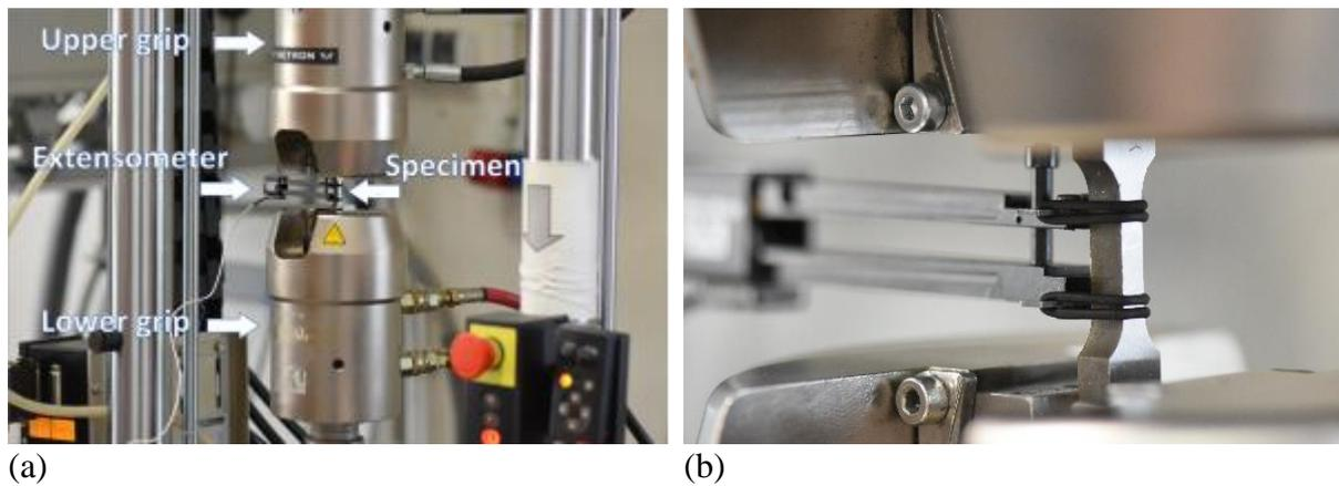
Fig. 7. Mini-specimen in grips of the 8874 Instron servo-hydraulic testing machine before a tensile test: (a) general view, (b) specimen and 2620-601 Instron uniaxial extensometer
