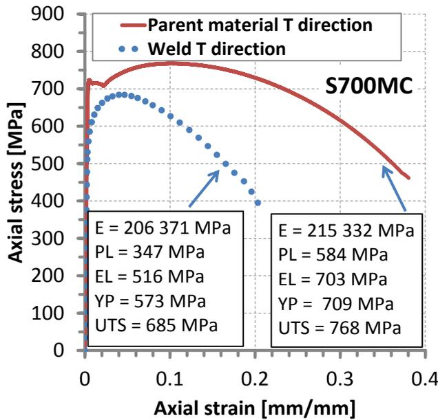
Fig. 11. Tensile characteristics of the parent material and its weld determined by means of specimens selected from the transverse direction
