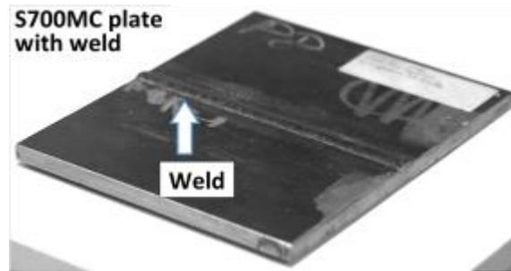
Fig. 3. The S700MC high strength steel plate with a weld
