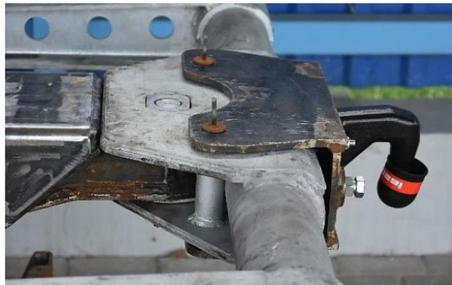
Fig. 1. The coupling zone made of the S700MC high-strength steel
