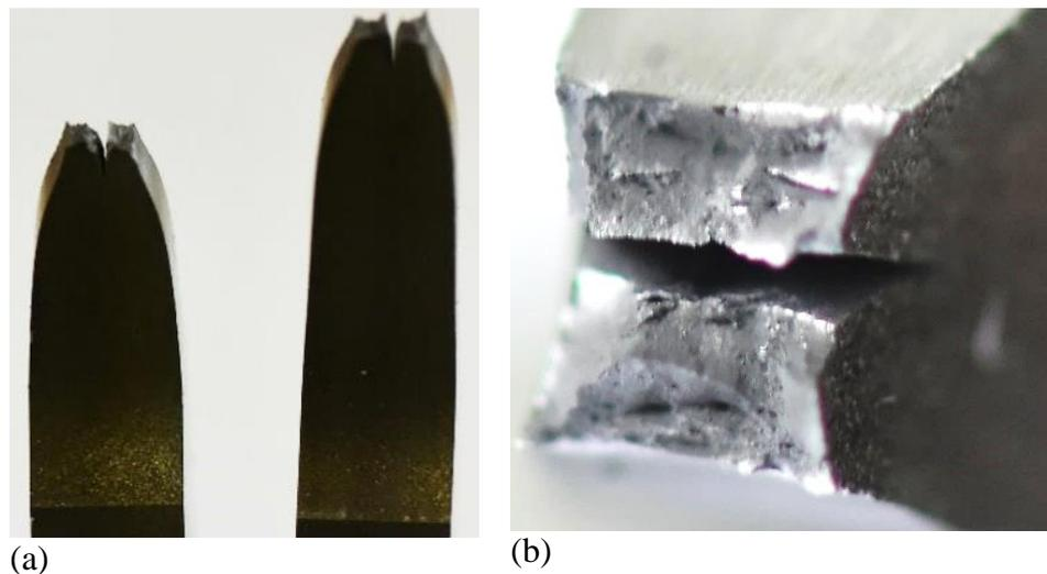
Fig. 15. Fracture zones of the HAZ
