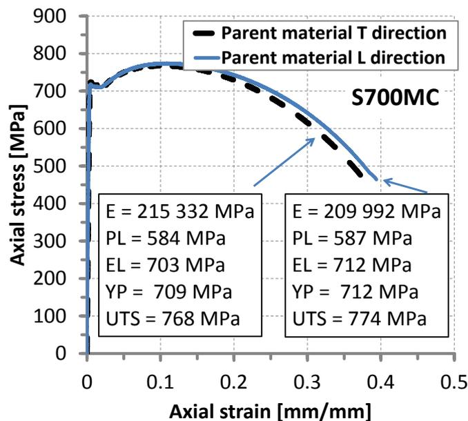
Fig. 9. Tensile characteristics of the parent material selected from both directions, i.e. longitudinal (L) and transverse (T), E – Young's modulus, PL – proportional limit, EL – elastic limit, YP – yield point, UTS – ultimate tensile strength
