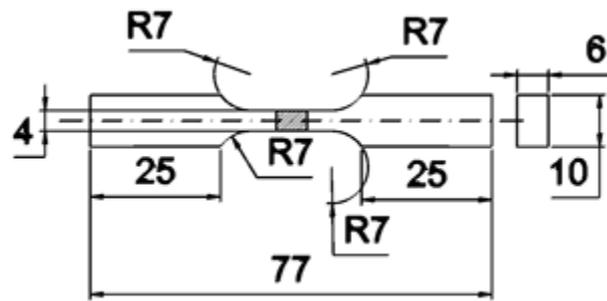
Fig. 5. Mini-specimen used for the parent material and its weld testing under monotonic tensile conditions
