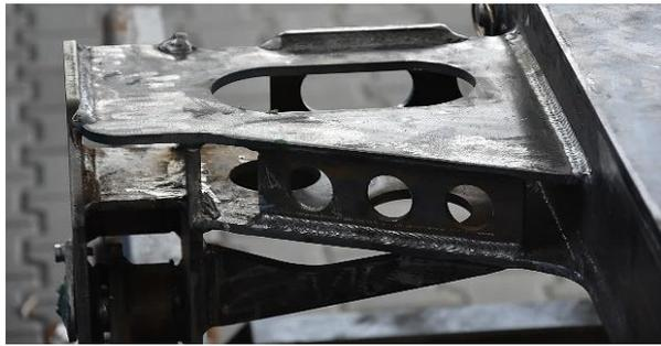
Fig. 2. Support of a towing boom body made of the S700MC high-strength steel for the recovery vehicle
