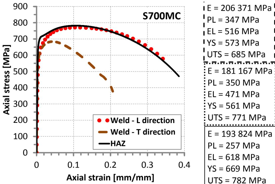
Fig. 12. Tensile characteristics of the weld and HAZ
