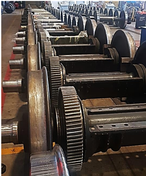
Fig. 1. Examples of gear applications in rail vehicles: a) fragment of the wheelset gearbox, b) example of gearbox used in the construction of locomotive engine
