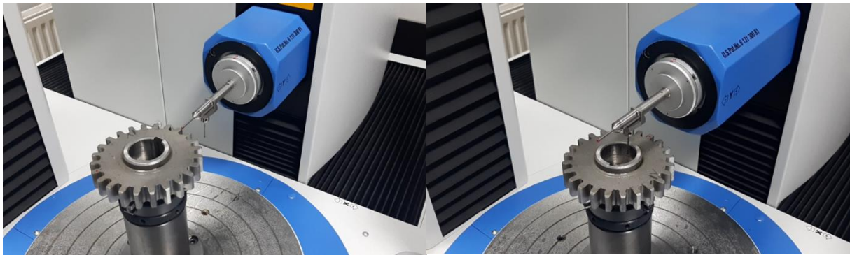
Fig. 2. Klingelnberg GmbH test stand used during measurement of selected geometrical parameters
