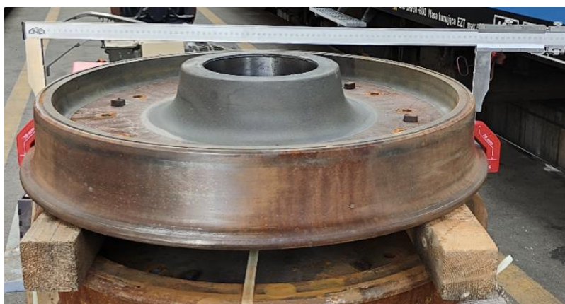
Fig. 7. View of the vernier calliper measurement with measurement bases
