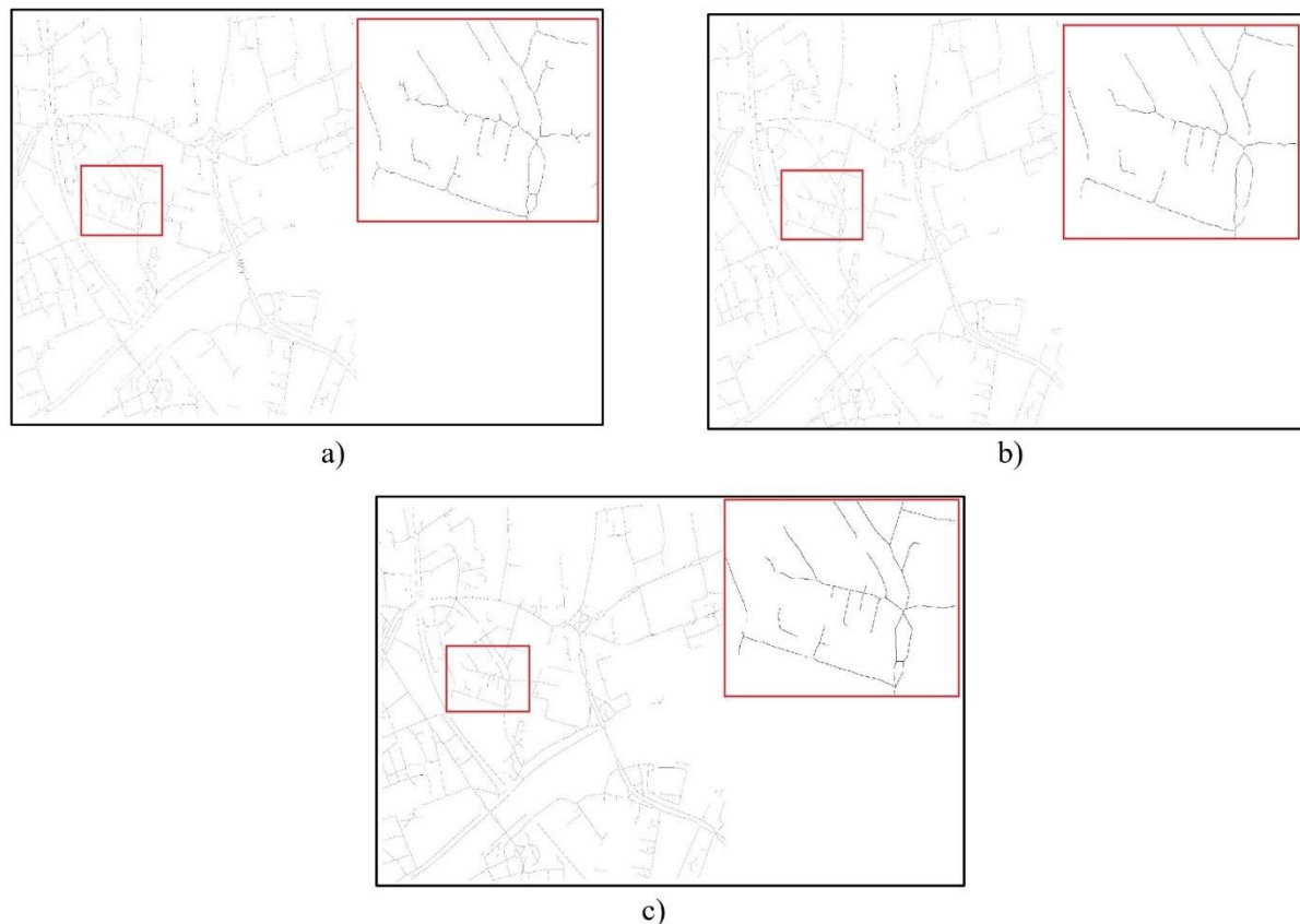
Fig. 6. The resulting raster with the detected road network – detection of road axes, by various methods: a) thinning, b) skeletonization, c) automatic vectorization
