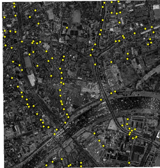
Fig. 2. Distribution of points representing roads on the intensity raster
