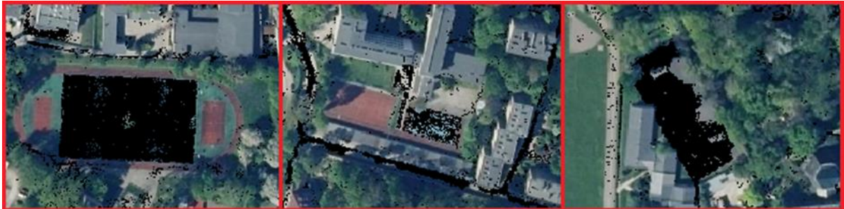
Fig. 4. Examples of incorrectly detected surface elements (playfields, parking)
