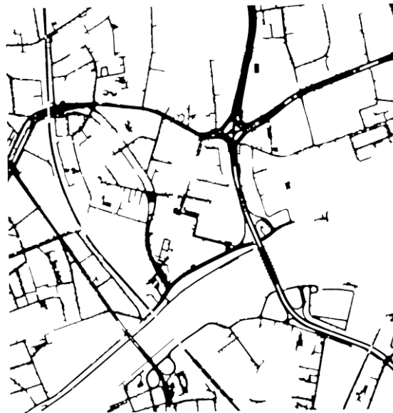
Fig. 5. The resulting raster with the detected road network
