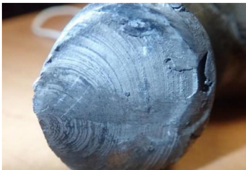
Fig. 12. Fatigue fracture of a chain link [8]
