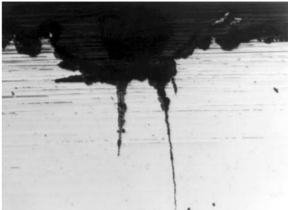
Fig. 9. An example of a corrosion pit on a cross-section through the parent material of a chain link [8]
