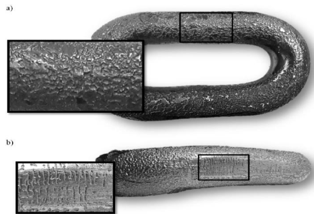
Fig. 10. Chain link corrosion: a) surface pitting, b) fatigue cracks intensified by corrosive environment [11]
