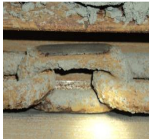
Fig. 8. Link abrasion on the conveyor trough [15]
