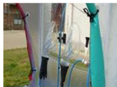
Fig. 10. Service gloves of transparent material installed in the window
