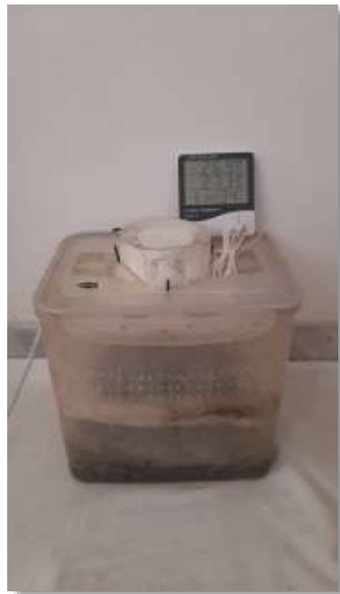
Fig. 8. Porous asphalt evaporation measuring device
