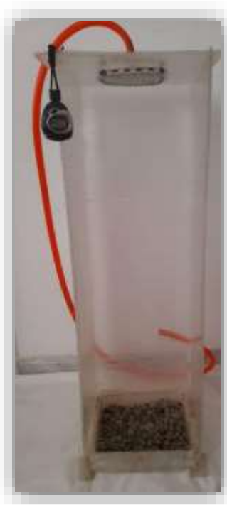
Fig. 6. Porous asphalt penetration measuring device with rain simulation
