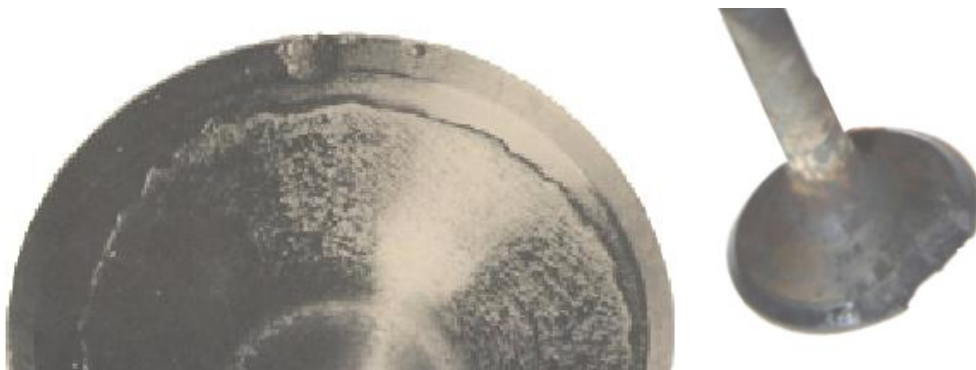
Fig. 1. Examples of valve damage resulting from carbon deposits [14]
