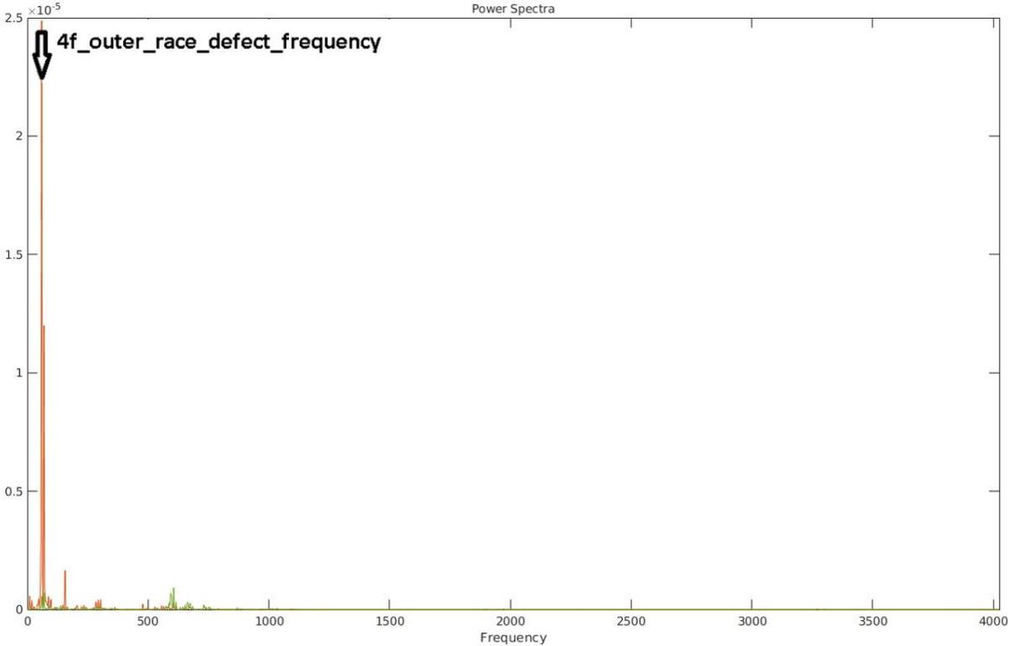
Fig. 10. Analysis of the vibration time-frequency waveforms - comparison of signals with new and damaged bearing - where green line indicates a new bearing, red line indicates a damaged bearing
