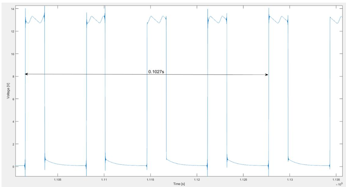
Fig. 3. Time course of the wheel speed signal - dynamic balancer
