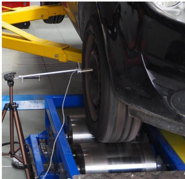
Fig. 7. Prototype stand during tests of the technical condition of the road wheel bearing hub
