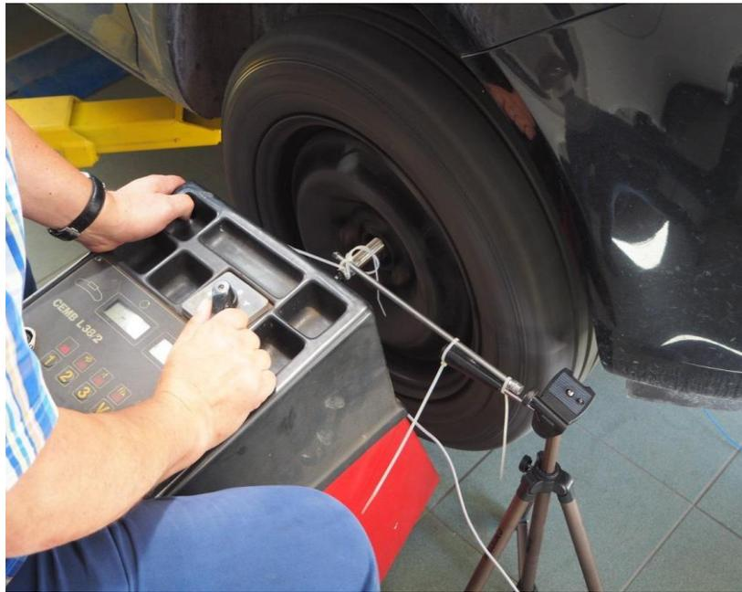
Fig. 2. Measurement stand during tests
