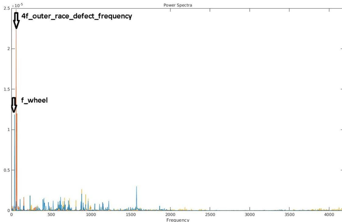
Fig. 8. Analysis of time-frequency waveforms of vibration signals of a wheel with a damaged rolling bearing - prototype stand – where: blue line - X-axis, red line - Y-axis, yellow - Z-axis
