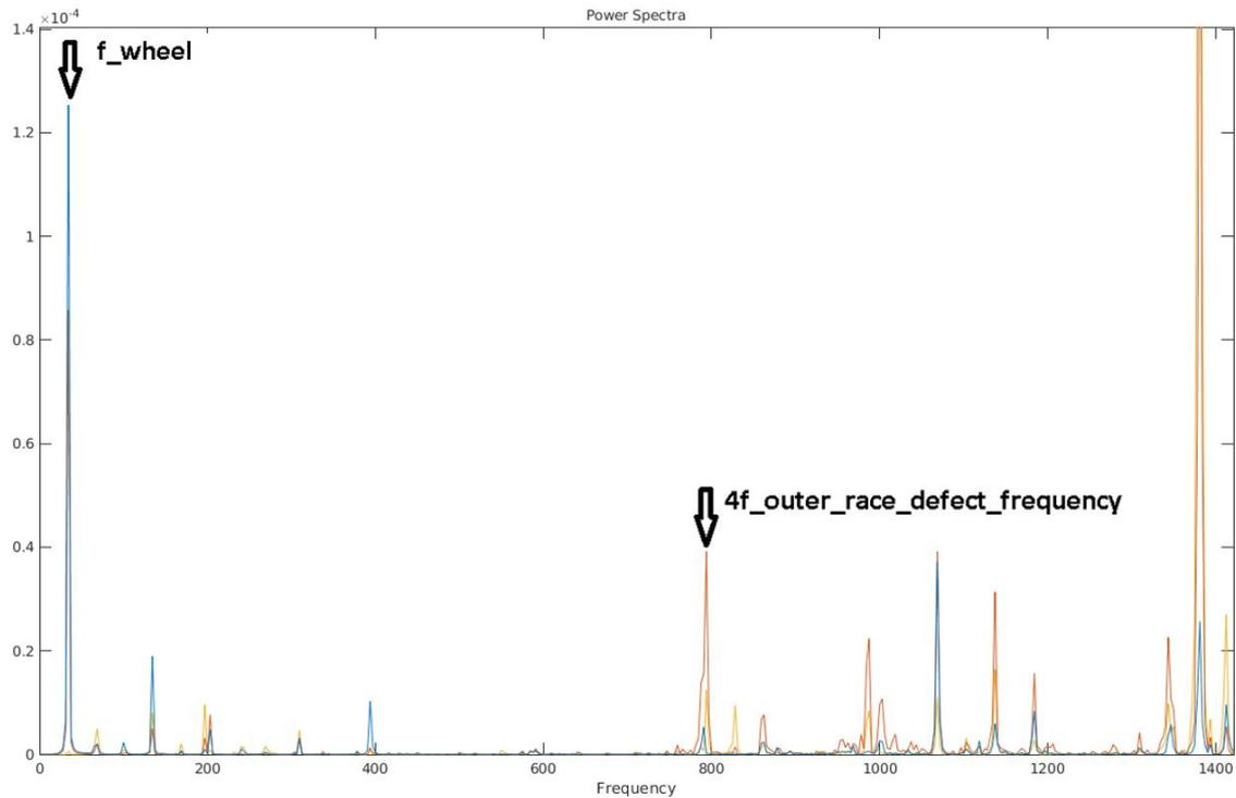
Fig. 4. Analysis of vibration signal waveforms of a wheel with a damaged rolling bearing - dynamic balancer – where: blue line - X-axis, red line - Y-axis, yellow - Z-axis
