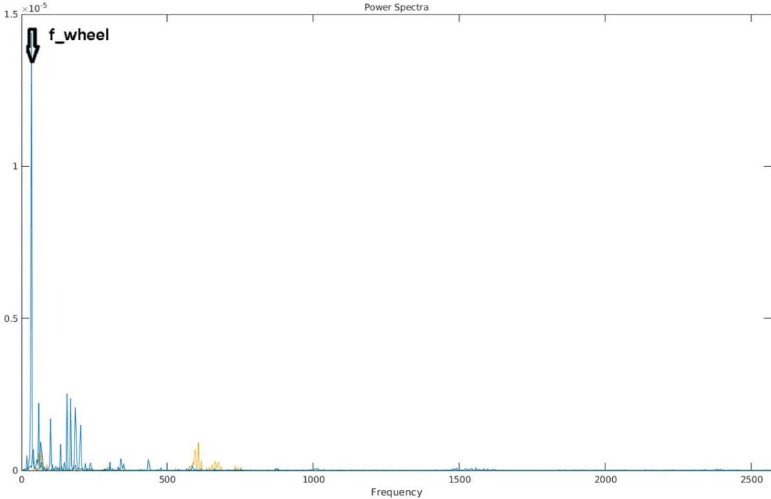
Fig. 9. Analysis of time-frequency waveforms of vibration signals of a wheel with a new rolling bearing-where: blue line - X-axis, red line - Y-axis, yellow - Z-axis
