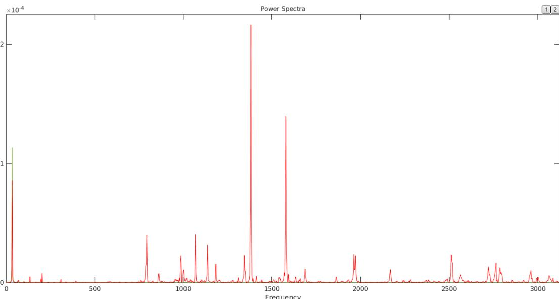
Fig. 6. Analysis of the time-frequency waveforms of the road wheel - comparison of a new and a damaged bearing - where green line indicates a new bearing, red line indicates a damaged bearing
