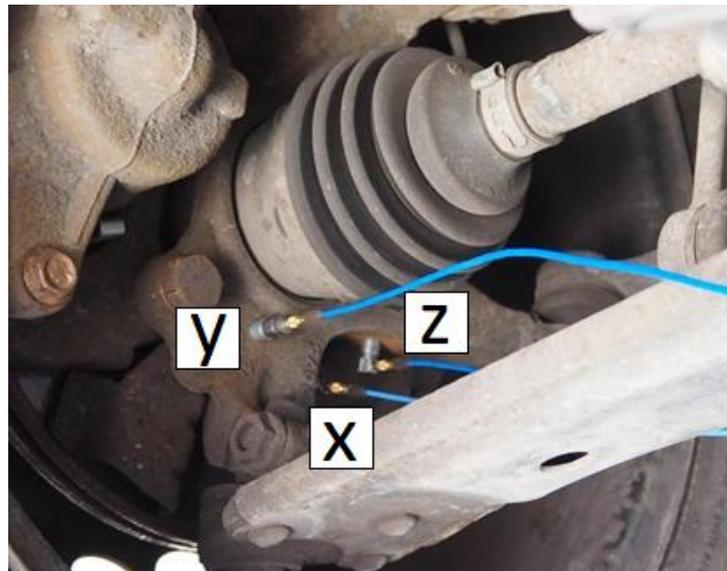
Fig. 1. View of placing vibration acceleration sensors on the wheel hub of the tested vehicle
