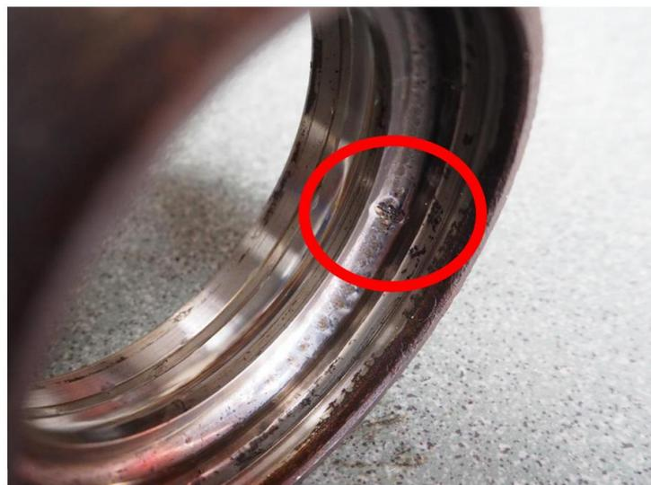
Fig. 11. View of damage to the outer race of the rolling bearing of the tested vehicle
