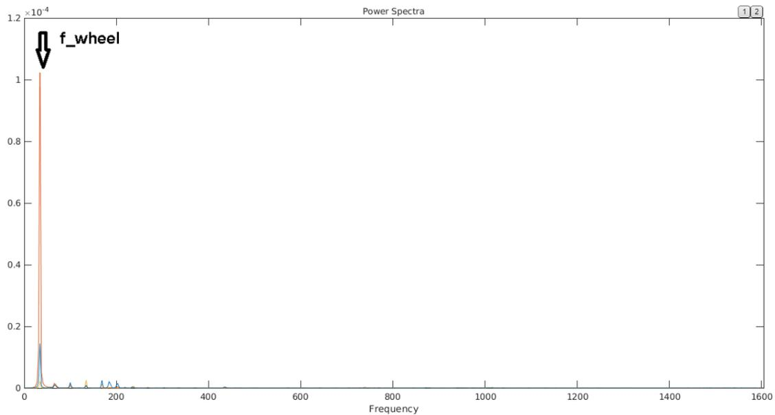
Fig. 5. Analysis of time-frequency waveforms of vibration signals of a wheel with a new rolling bearing – where: blue line - X-axis, red line - Y-axis, yellow - Z-axis
