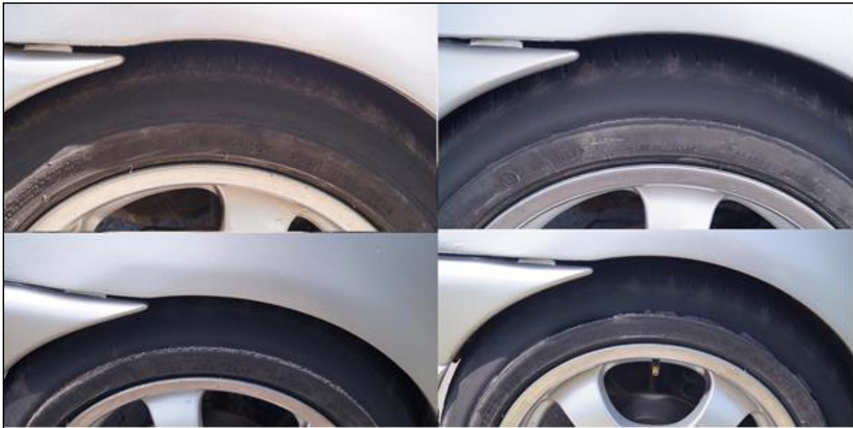
Fig. 10. Phases of damage to the Bridgestone Turanza ER300 tyre sidewall during the tests Source: authors' study
