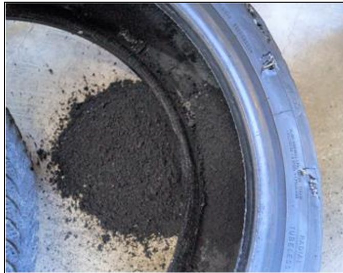
Fig. 12. View of the destroyed rubber collecting inside the tyre while driving at a pressure of 0 kPa Source: authors' study
