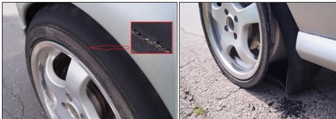
Fig. 11. View of the process of cutting the sidewall of the Bridgestone Turanza ER300 tyre while covering the test distance: on the left, the initial phase of the belting damage on the right, complete cutting of the sidewall of the tyre Source: authors' study
