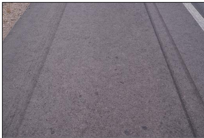
Fig. 14. View of the emergency braking marks (blocked wheels) for the Run Flat Bridgestone Turanza ER300 RFT tyre with a pressure of 0 kPa (right) and the road tyre (left)
