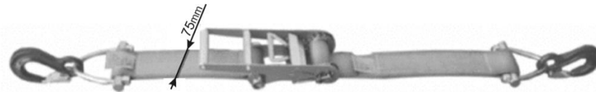
Fig. 12. Fastening strap used for lashings S_3, S_3' and S_4, S_4'
