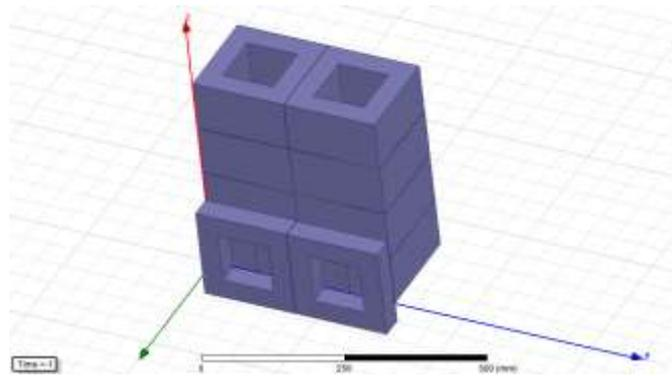
Fig. 2. Moving coils in front of acceleration stages
