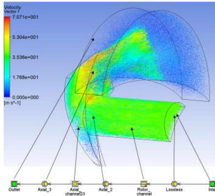
Fig. 2. Axial intake port 3D calibration
