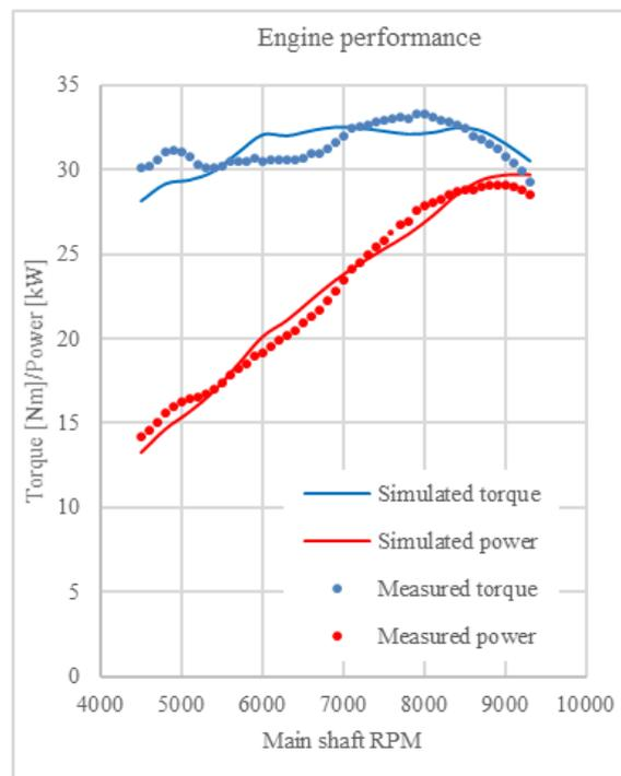
Fig. 3. Engine prediction correlation with measured data
