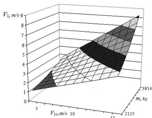
Fig. 6. Dependence after-the-shock velocity on the operational factors at the third phase
