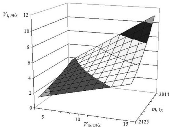
Fig. 4. Dependence after-the-shock velocity on the operational factors at the first phase
