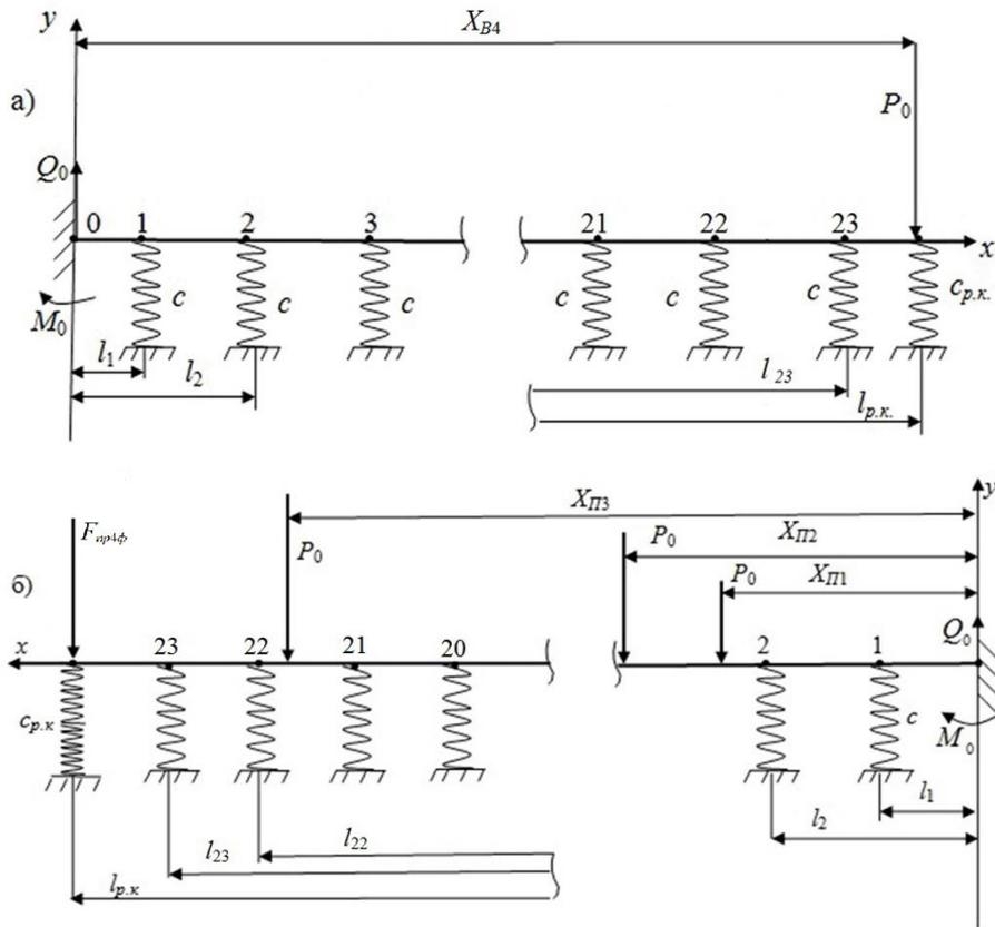
Fig. 2. The mechanical pattern of calculation of the junction height in the fourth motion phase: a) rear rail; b) receiving rail
