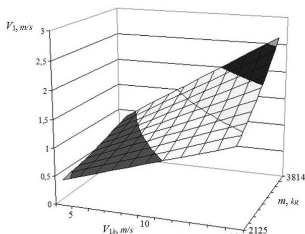
Fig. 7. Dependence after-the-shock velocity on the operational factors at the fourth phase
