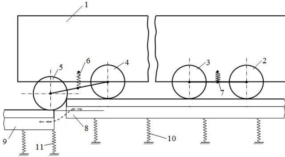
Fig. 1. The scheme of passage of butt roughness
