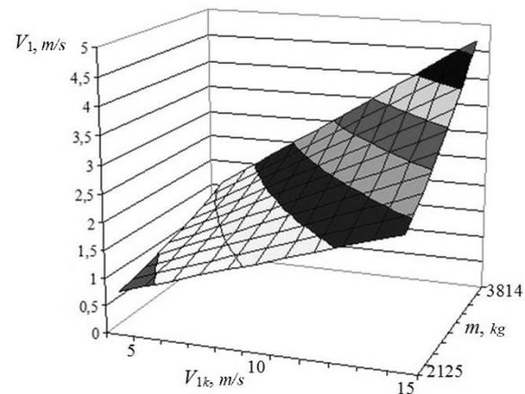
Fig. 5. Dependence after-the-shock velocity on the operational factors at the second phase
