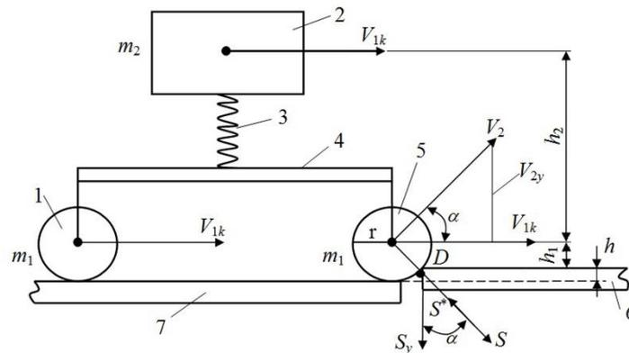
Fig. 3. Shock interaction scheme
