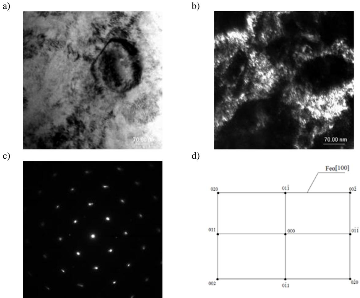
Fig. 8. Structure of the steel 50S2 from the used fastener: a) bright field, b) dark field, c) SAD electron diffraction pattern, d) solution of the electron diffraction,  $Fe_{\alpha}$  phase, zone axis [100]
