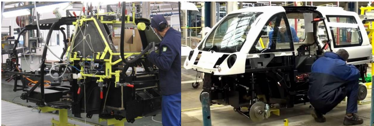
Fig. 4. The metal structure of the Mia Electric vehicle [17]
