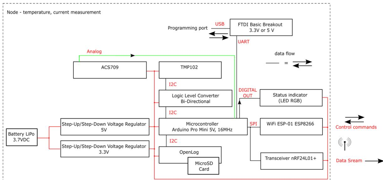
Fig. 7. Measuring node: temperature, current
