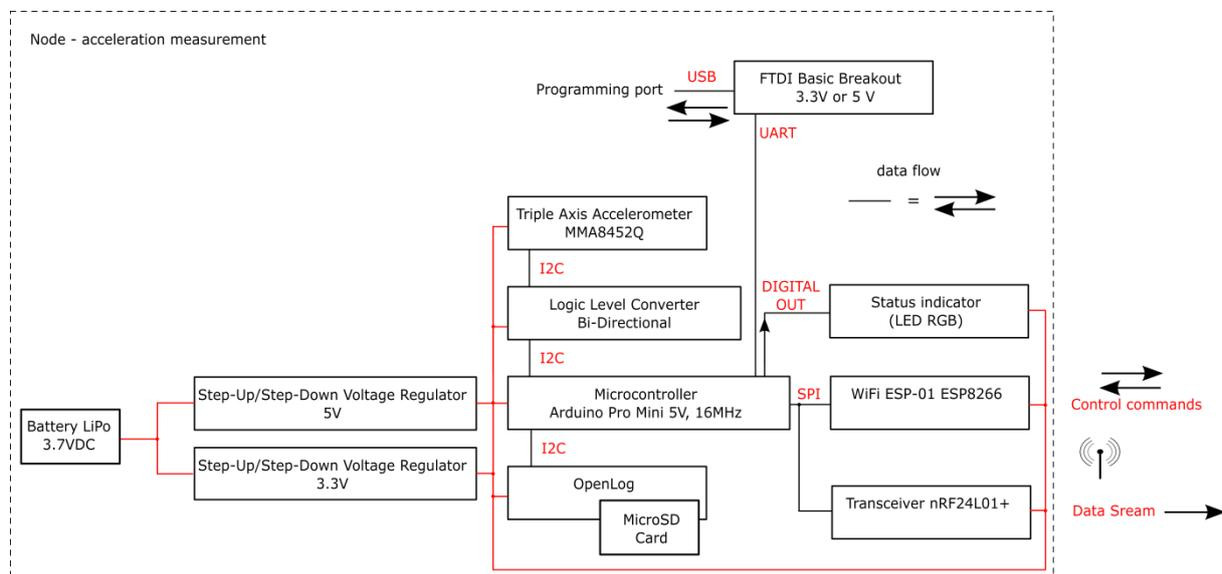
Fig. 9. Measuring node: acceleration
