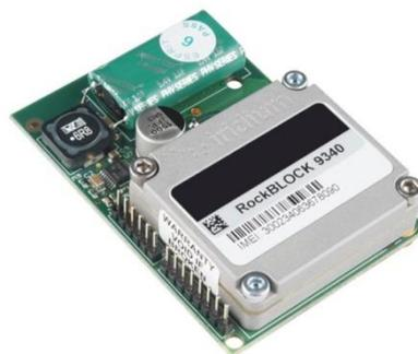
Fig. 5. RockBLOCK Mk2 Iridium SatComm Module [7]
