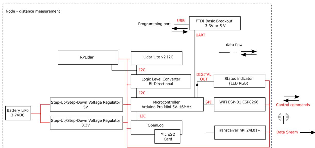
Fig. 11. Measuring node: distance, obstacles
