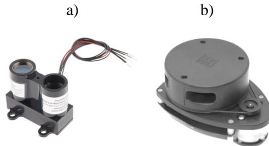
Fig. 12. a) Distance measurement: LIDAR-Lite [10] and
