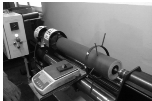
Fig. 3. The laboratory stand for the measurement of rollers dynamic resistance: 1 – load carrying structure, 2 – electrical engine, 3 – belt transmission, 4 – drive shaft support, 5 – clamp shaft support, 6 – roller, 7 – electronic balance, 8 – roller clamping ring, 9 – lever
