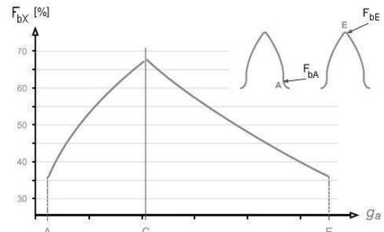
Fig. 2. Shape of the curves represents the load along the path of contact in one pair of HCR gearing teeth
