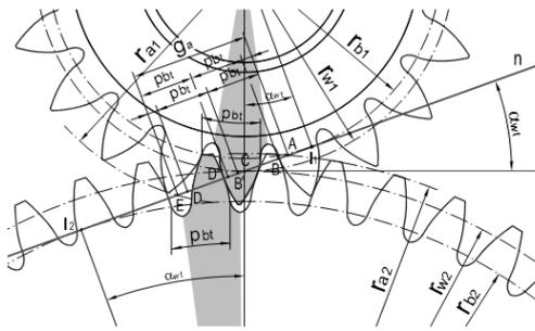
Fig. 1. Geometry of involute HCR gearing
