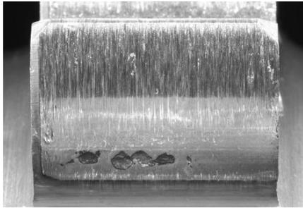
Fig. 4. Pitting in the HCR gearing
