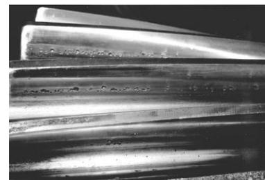
Fig. 3. Standard gear pitting damage
