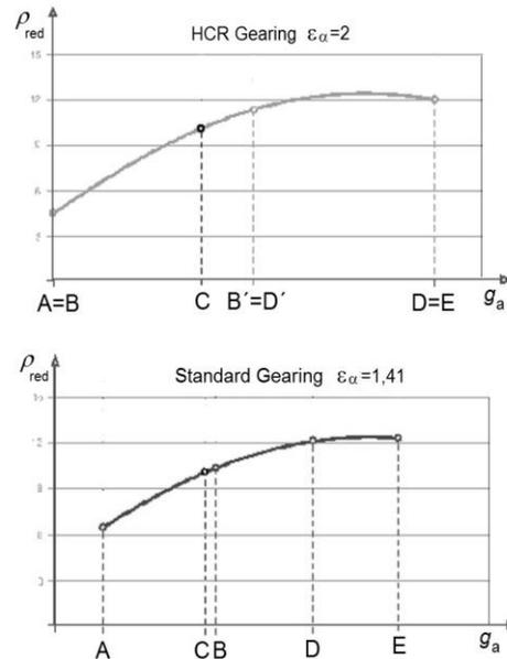
Fig. 5. Mean contact radius of curvature along the contact path
