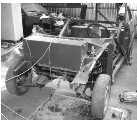
Rys. 5. Model zawieszenia Fiata Cinquecento wykorzystany w badaniach [9] Fig. 5. Fiat Cinquecento suspension model used in research [9]
