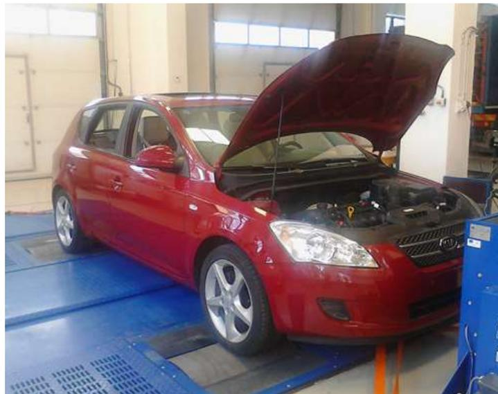
Fig. 2. Vehicle used for measuring and MAHA MSR 1050
