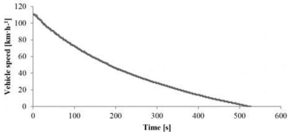
Fig. 3. Vehicle deceleration during coasting deceleration measurement
