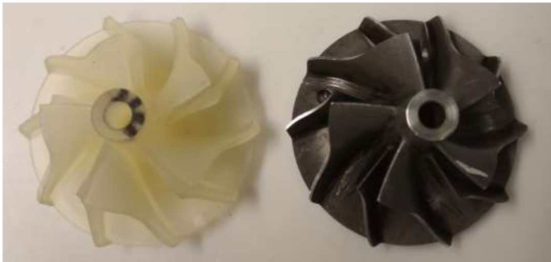
Fig. 2. Compressor wheel manufactured using the MJM method (left) and the original one (right)
