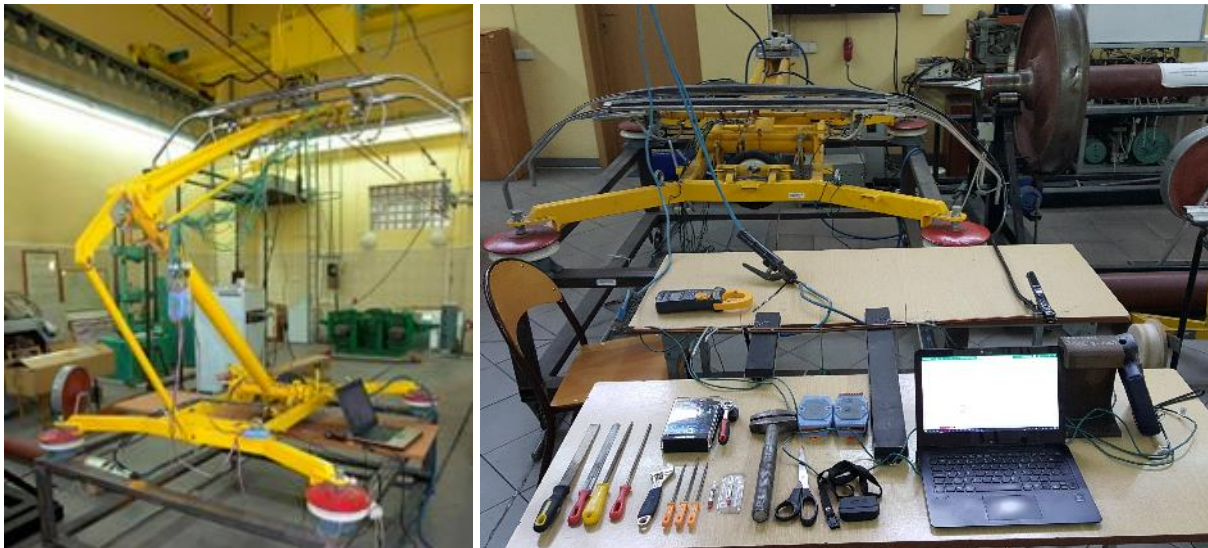
Fig. 1. Laboratory stand for pantograph and contact strip material testing
