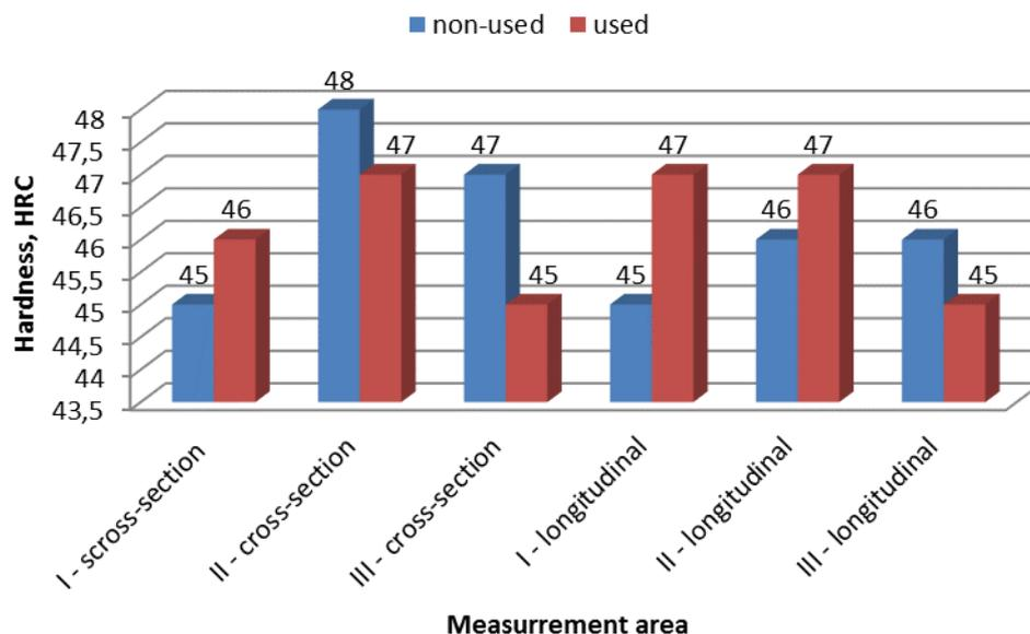
Fig. 9. Hardness measurement results for the chosen places of the fasteners
