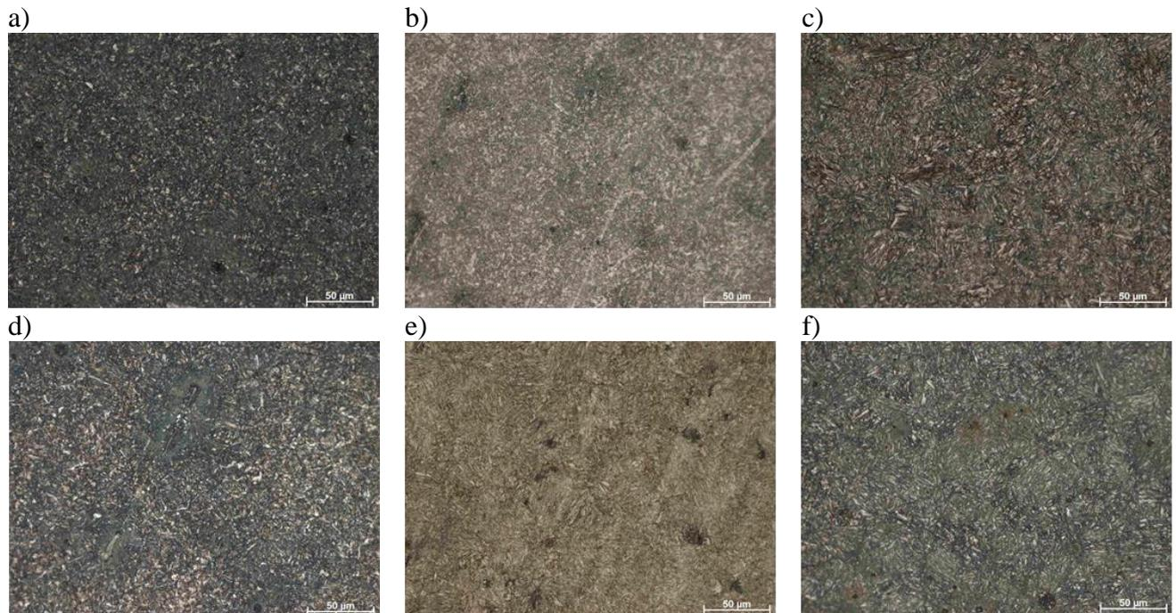
Fig. 4. Microstructure of the non-used: a), b), c) and used d), e), f) fasteners of the SKL 12 system, depending on the sampling place and direction, where: a) is from place no. I in Fig. 3a; b) is from place II in Fig. 3a and c) is from place III in Fig. 3a
