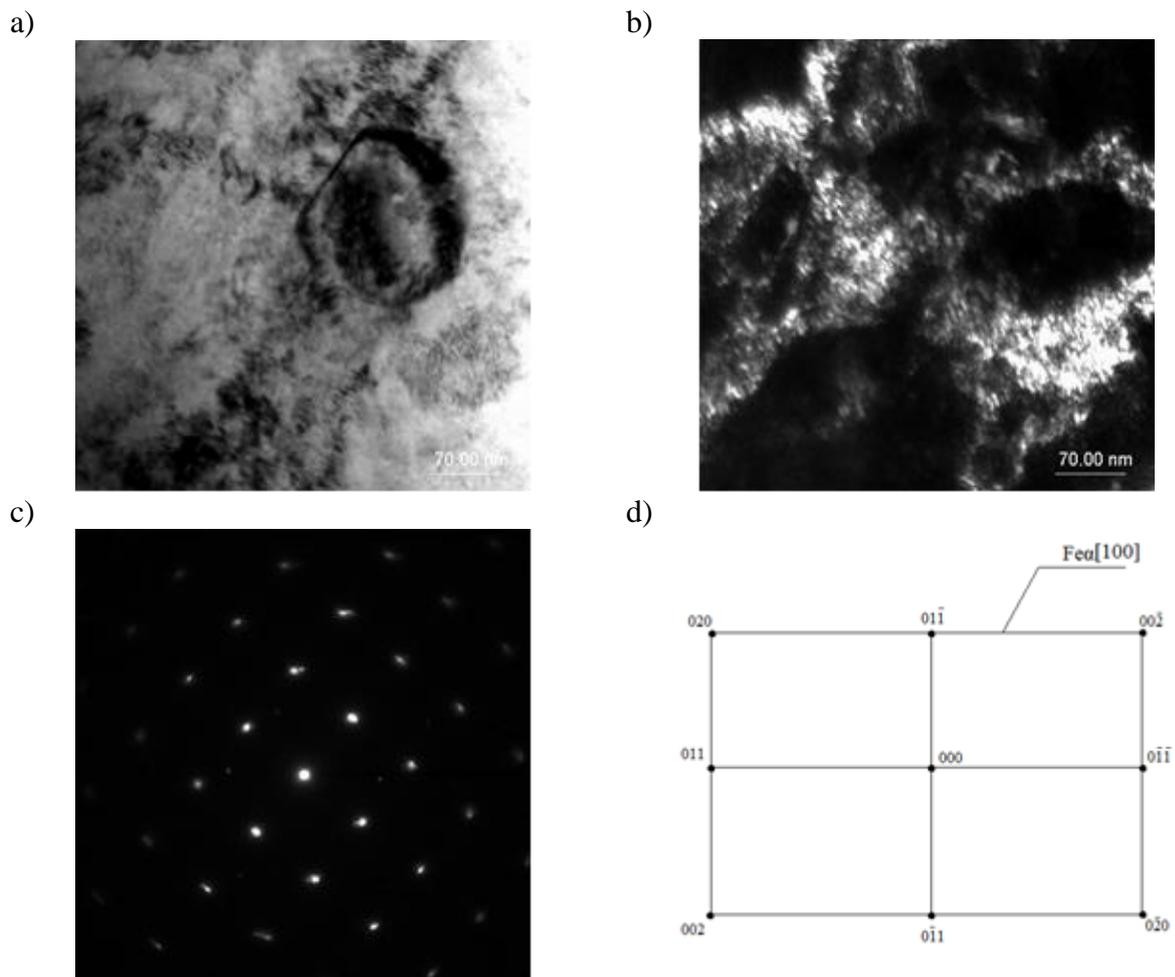
Fig. 8. Structure of the steel 50S2 from the used fastener: a) bright field, b) dark field, c) SAD electron diffraction pattern, d) solution of the electron diffraction,  $\text{Fe}_\alpha$  phase, zone axis [100]
