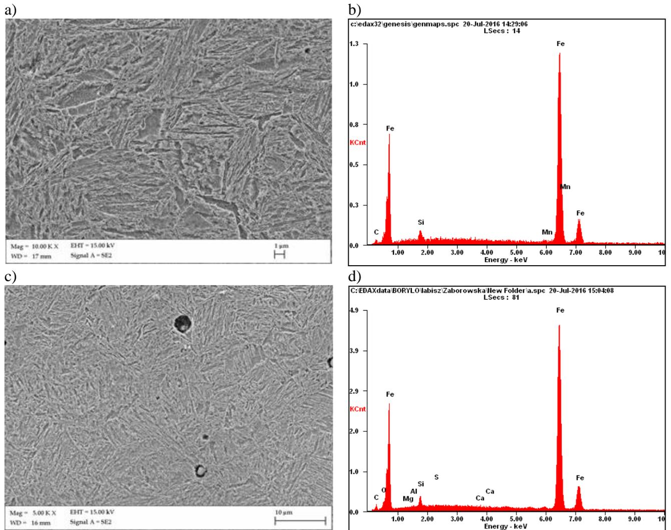
Fig. 6. Microstructure and the corresponding EDS area microanalysis of the non-used: a), b) and used c), d) fastener microstructure, carried out in point III (Fig. 3a), SEM
