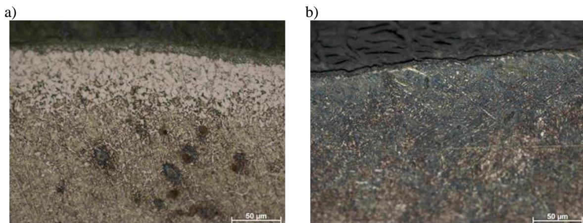
Fig. 5. Microstructure in the cross-section of the surface layer of the non-used (a), and used fasteners (b)
