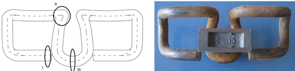
Fig. 3. The investigated fasteners of the SKL 12 system (a), places chosen for microstructure and hardness analysis (b)
