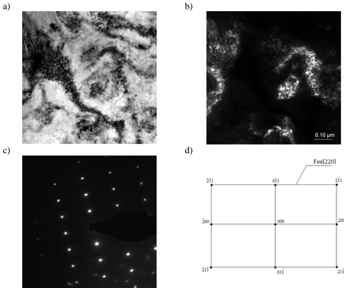
Fig. 7. Structure of the steel 50S2 from the non-used fastener: a) bright field, b) dark field, c) SAD electron diffraction pattern, d) solution of the electron diffraction,  $Fe_{\alpha}$  phase, zone axis [220]
