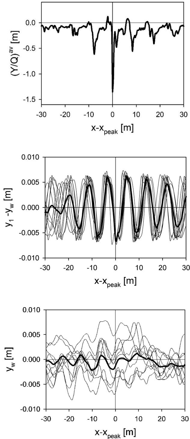
Fig. 1. Derailment coefficient  $Y/Q$ , lateral track irregularities  $y_w$  and relative lateral displacement of leading wheelset  $y_1 - y_w$  versus  $u = x - x_{\text{peak}}$  near various  $M = 10$  track points where the minima  $Y/Q \leq -1.3$  occur for the ride velocity  $v = 200$  km/h . The bold lines mark the average values  $y_w^{\text{av}}$ ,  $y_1^{\text{av}} - y_w^{\text{av}}$ ,  $(Y/Q)^{\text{av}}$  ; Equations 1 and 2)
