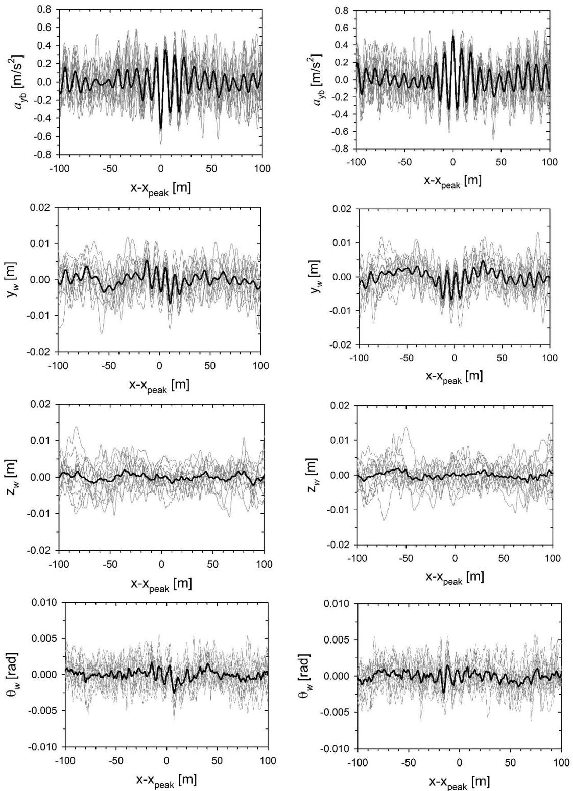
Fig. 2. Lateral body acceleration  $a_{yb}$  and track irregularities:  $y_w$ ,  $z_w$  and  $\theta_w$  (thin grey lines) around the points  $x_{\text{peak}}^{(k)}$  ( $k = 1, \dots, M = 13$ ) where  $a_{yb} < -0.45 \text{ m/s}^2$  (left column) or  $a_{yb} > 0.45 \text{ m/s}^2$  (right column) and their averages  $a_{yb}^{\text{av}}$ ,  $y_w^{\text{av}}$ ,  $z_w^{\text{av}}$ ,  $\theta_w^{\text{av}}$  (thick black lines) for  $v = 160 \text{ km/h}$
