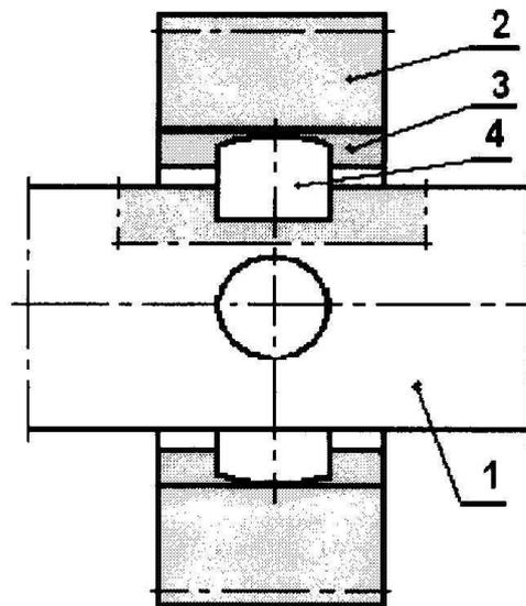
Fig. 2. Diagram of oscillating wheel setting on the shaft, using four cylinders. Description of indications: 1) shaft's journal; 2) toothed gear; 3) groove with rectangular cross section; 4) cylinder [10]
