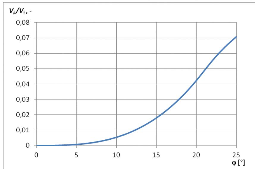
Fig. 6. Graph of  $V_k/V_f$  ratio as a function of the angle of hub deflection  $\phi$
