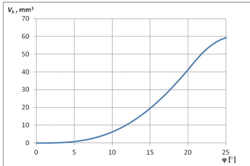
Fig. 4. Overlapping volume  $V_k$  diagram as a function of angle  $\phi$  between the journal axis and the hub axis
