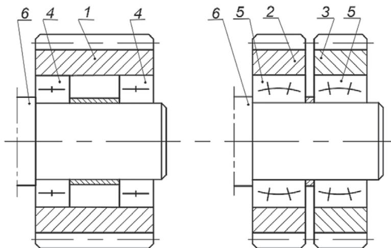
Fig. 1. Diagram of a portion of a satellite wheel with bearing. Description of indications:
