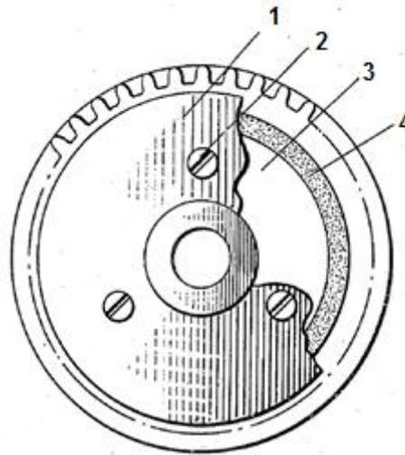
Fig. 7. Scheme of construction of wheel with a malleable ring. Description of indications:
