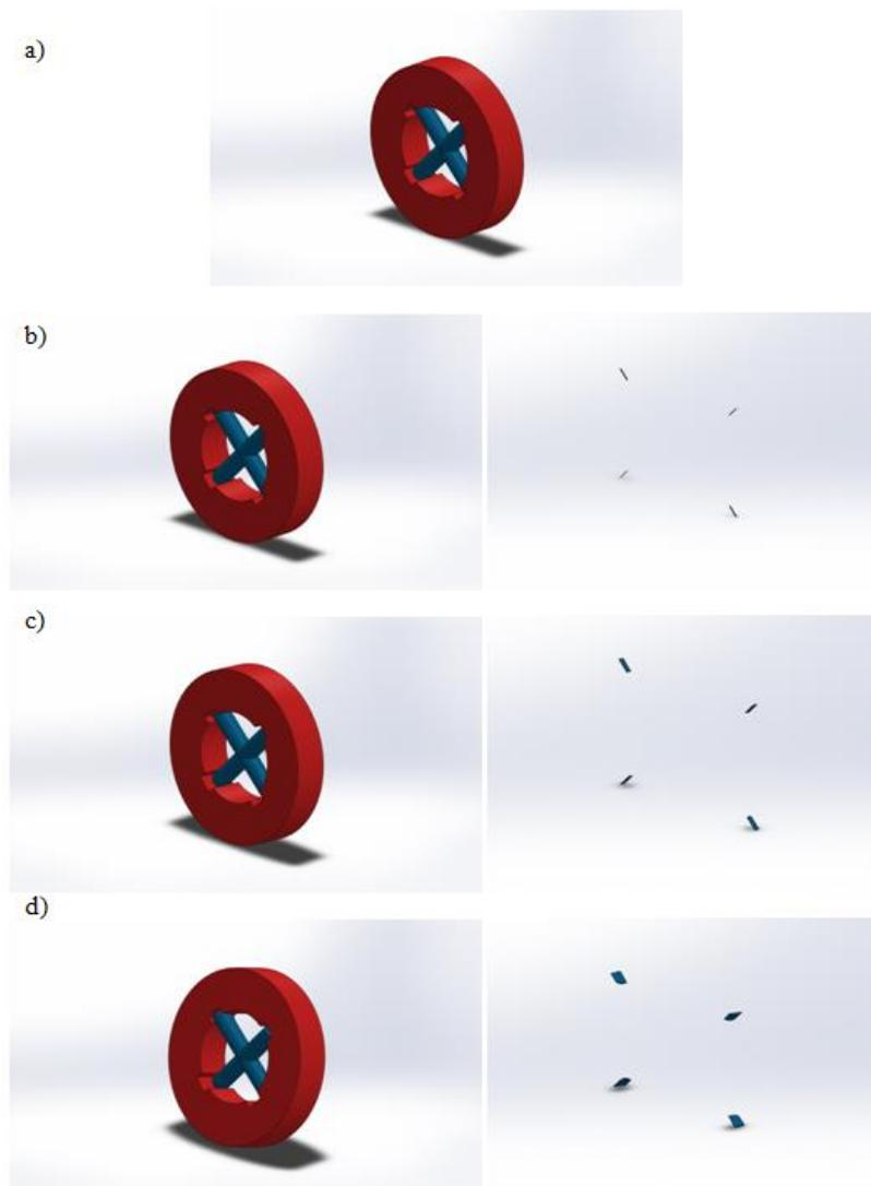
Fig. 3. Simulation of the hub oscillating operation: a) three-dimensional model of the joint showing the main characteristics of the analysed solution; b) the angle between the journal axis and the hub axis is  $1^\circ$ ; c) the angle between the journal axis and the hub axis is  $5^\circ$ ; d) the angle between the journal axis and the hub axis is  $15^\circ$
