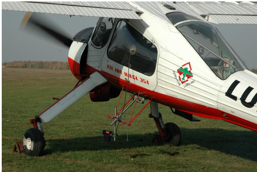
Fig. 2. The PZL 104 Wilga 35A, a typical STOL airplane (note the rocker arm-type wheel suspension on the main landing gear)
