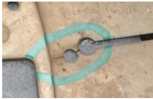
Fig. 3. Crack in the brake pressure plate Source: author's ABT Košice wheel and brake shop
