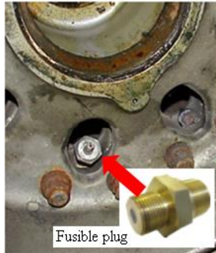
Fig. 2. Fusible plug on the wheel disc
