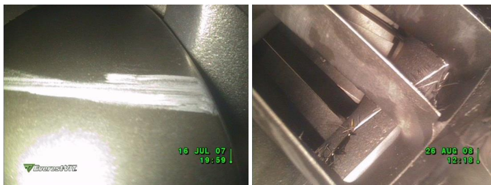
Fig. 1. Evidence of a bird strike
