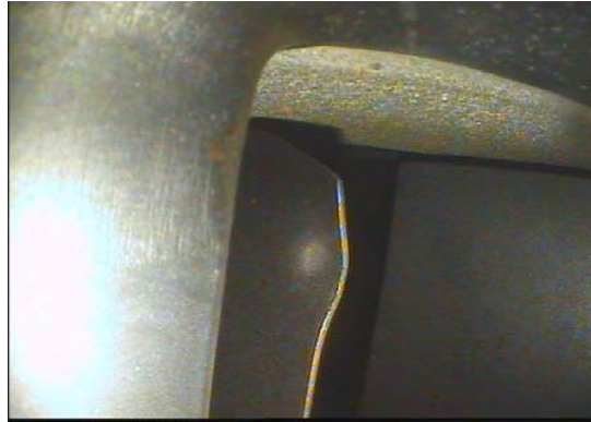
Fig. 2. Low-pressure compressor's trailing edge blade bend
