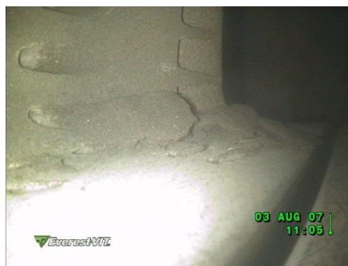
Fig. 6. Chunks of surface coating at the trailing edge of a high-pressure turbine blade
