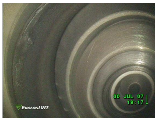
Fig. 4. Minor carboning on the fuel nozzle
