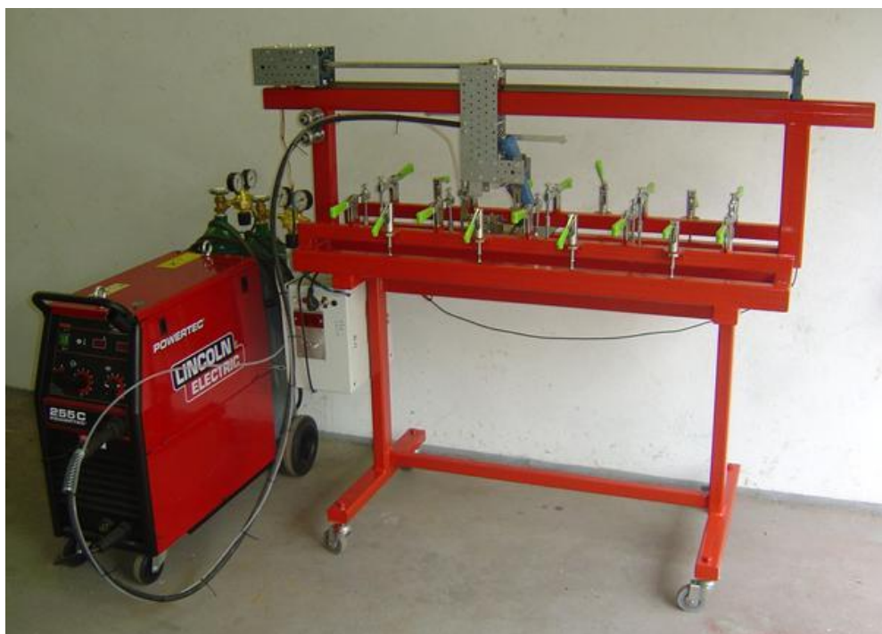
Rys. 3. Aparat do spawania mikrojetowego Fig. 3. Apparatus for welding with micro-jet cooling
