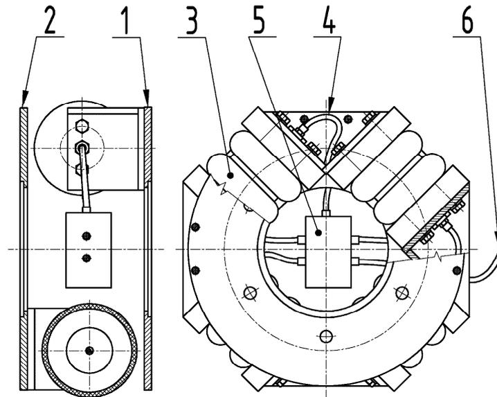
Fig. 3. Pneumatic flexible coupling type 4-2/70-T-C
