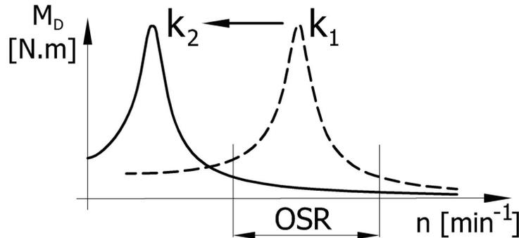
Fig. 1. Principle of mechanical systems tuning
