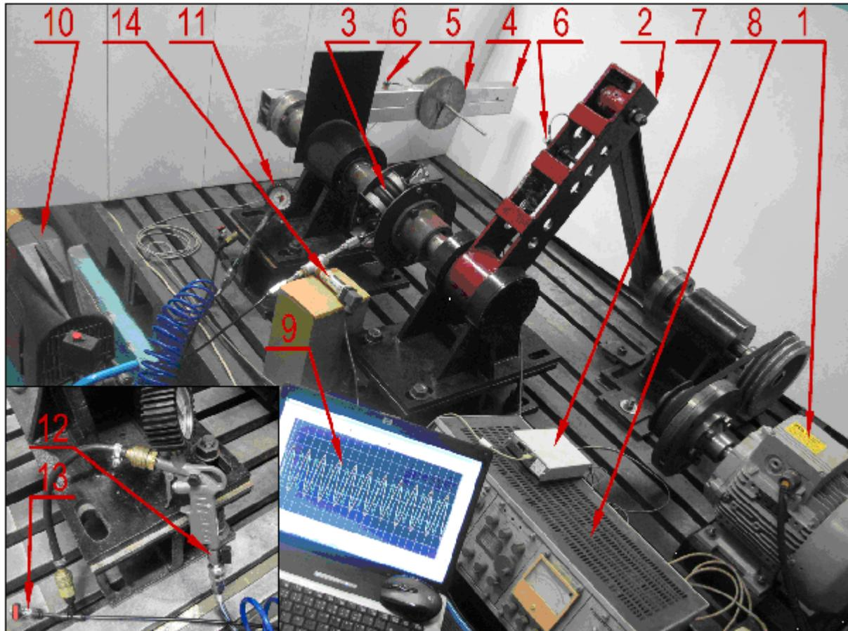
Fig. 2. Examined torsional oscillating mechanical system
