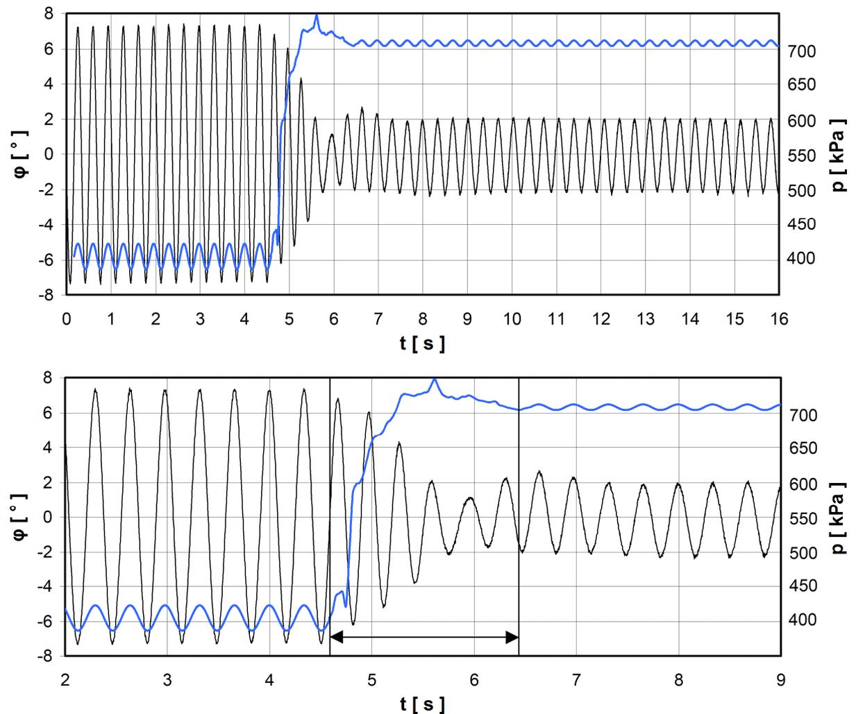
Fig. 10. Transitional effect from the resonance region at rapid air overpressure increase
