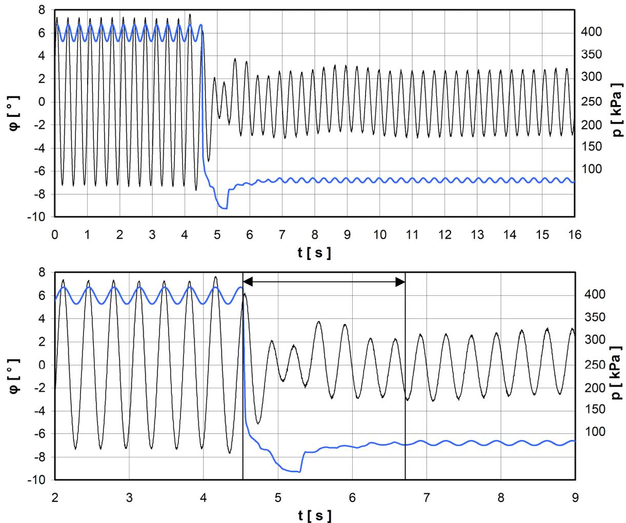
Fig. 11. Transitional effect from the resonance region at rapid air overpressure decrease
