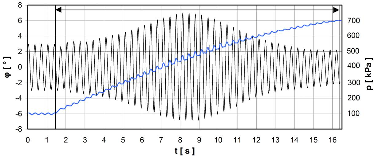
Fig. 7. Transitional effect across the resonance region at slow air overpressure increase
