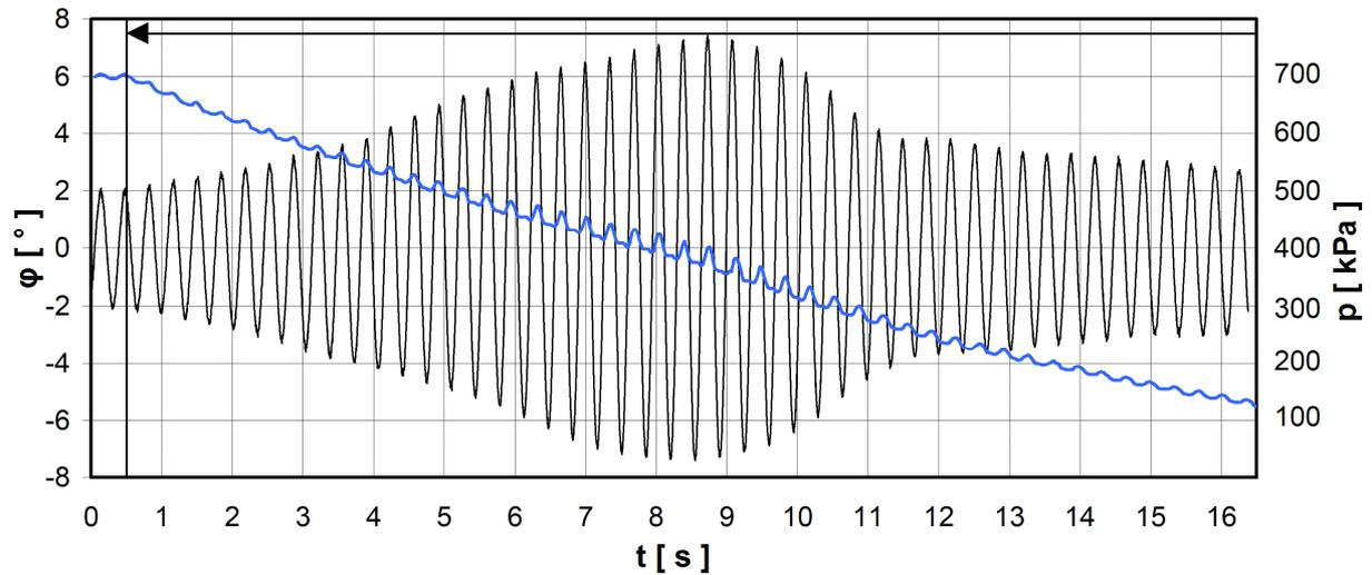
Fig. 9. Transitional effect across the resonance region at slow air overpressure decrease
