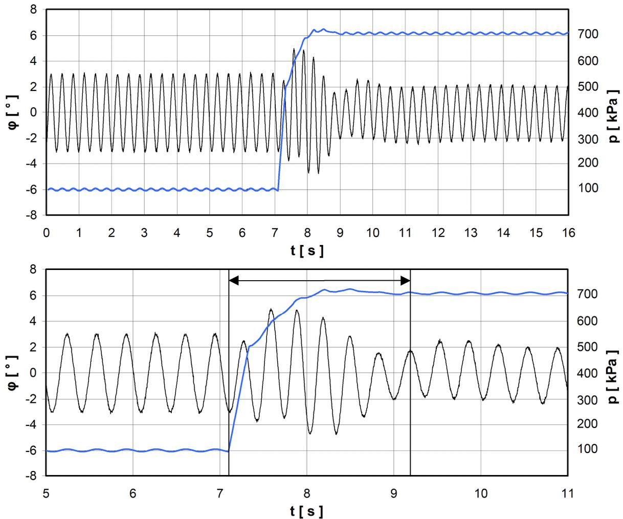
Fig. 6. Transitional effect across the resonance region at rapid air overpressure increase
